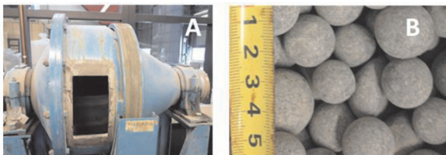
Figure 7-5: Applied lab-scale ball mill (A) and steel balls (B).
