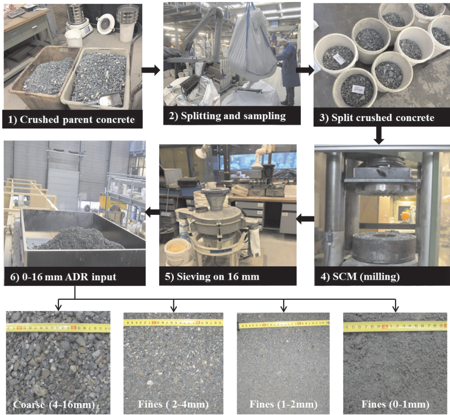
Figure 5-5: Different steps of the performed recycling process and final produced recycled fractions.
