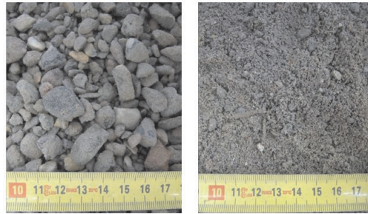
Figure 2-2: Products from crushed concrete by ADR: Coarse (left) and Fine (right)[5].
