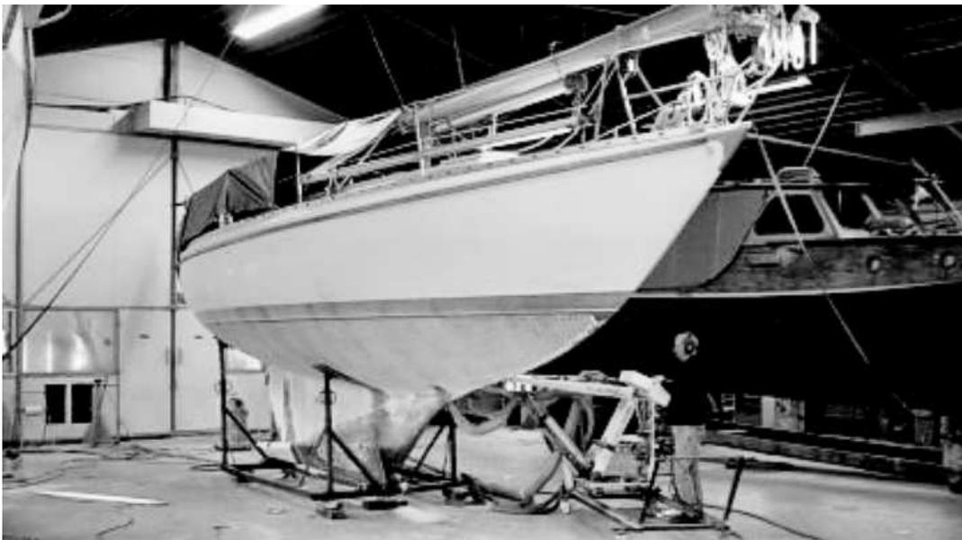
*Surface treatment of the bottom of a sailing boat, to prevent the growth of osmosis*
