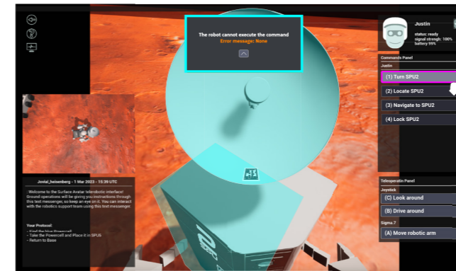
(1) Localize: The Object consists of multiple parts, the one on the bottom is not localized well, because the AprilTag is not fully in view. Moving the head to view the Tag better will help to localize it correctly.
