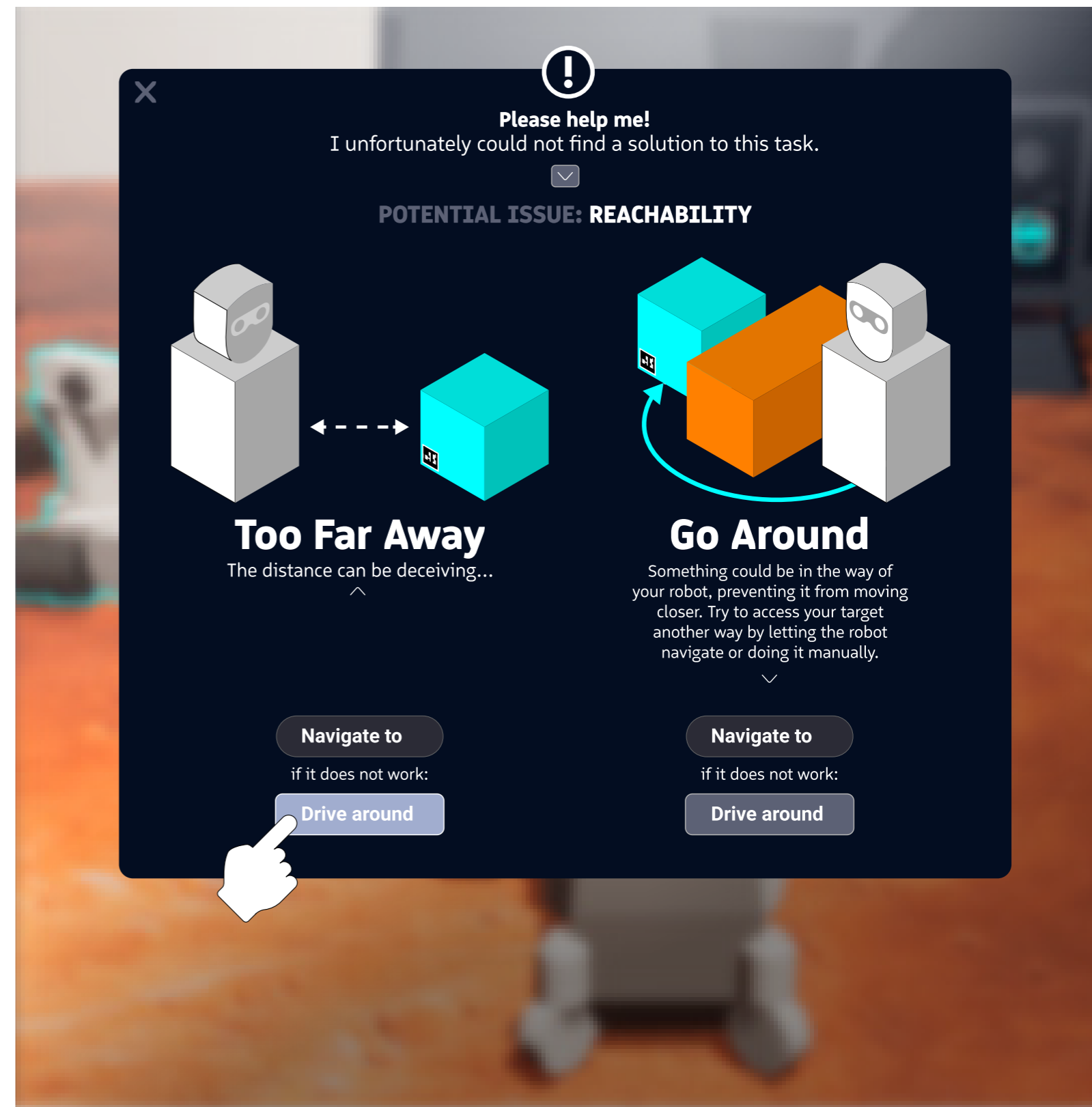
Figure 45: An example of an adapted "Typical Errors and Solutions" debug page showcasing enhancements such as expandable text for detailed explanations and direct command interaction. These improvements are integrated into the third-person perspective.
