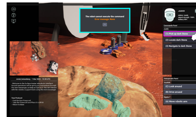
(2) Collision: The other stones in front of the one that the robot is trying to grab are causing a collision. Trying it again or simply approaching the desired Object from another position will help to grab it.
