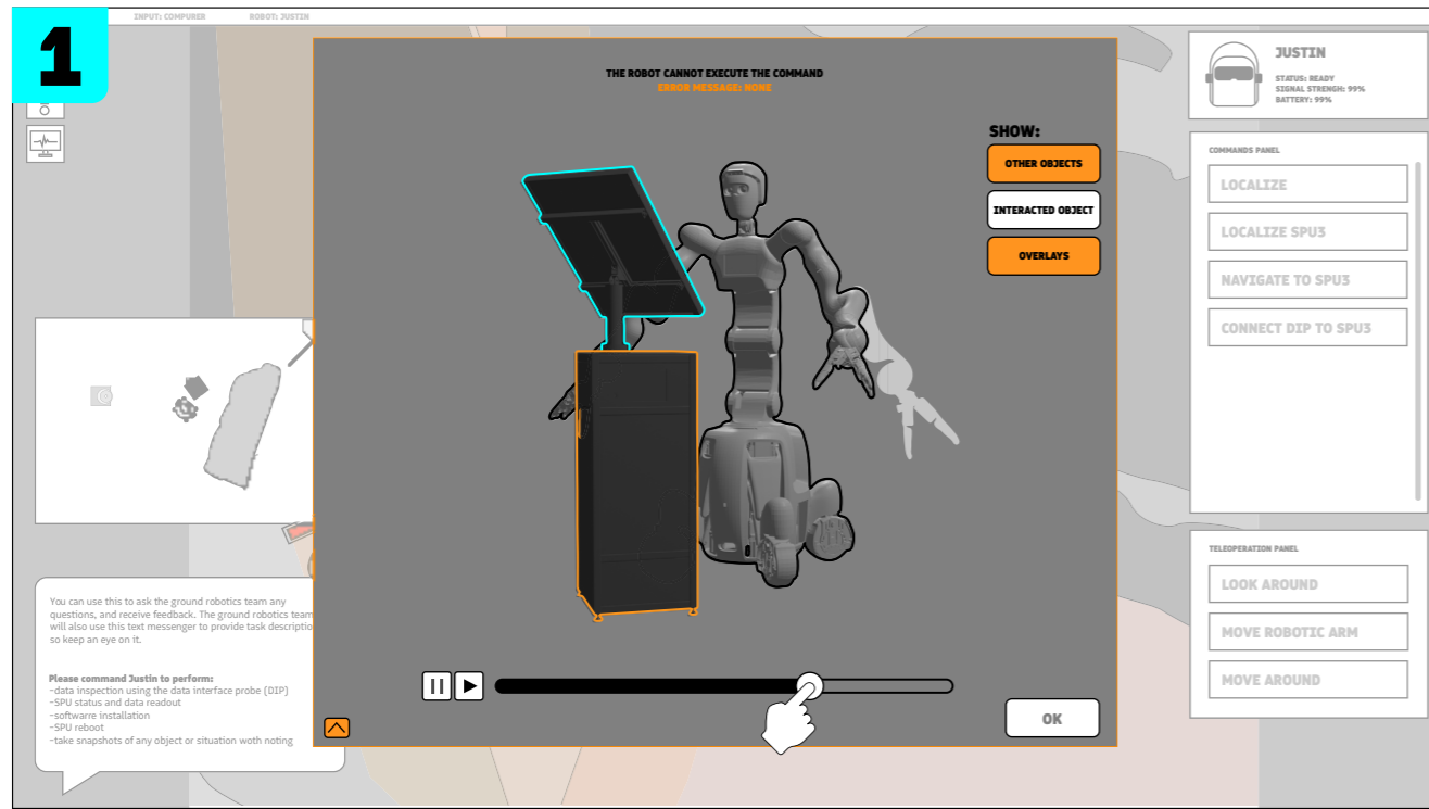
Figure 24: Overview of the Debugging Dashboard concept; (1) Motion planning, (2) Robot statistics, (3) Typical problems and solutions, (4) Motion plan flowchart with animation steps and (5) Motion plan flowcharts as graph
