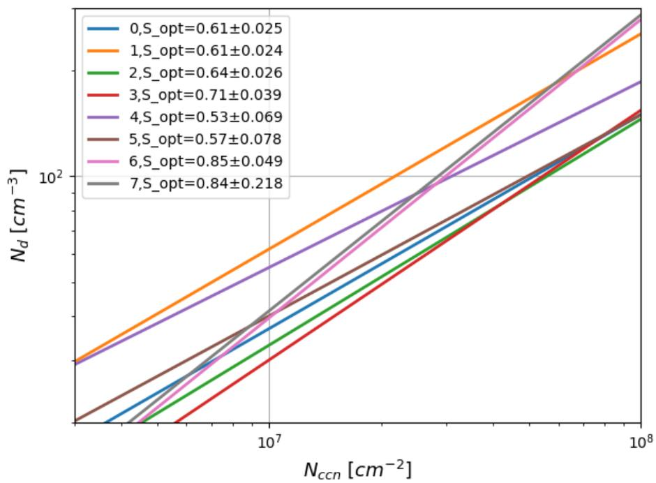
**Figure 3.18:** The computed least-squares fit to the binned satellite retrievals per cluster. The susceptibilities and the least-squares error are shown in the legend.
