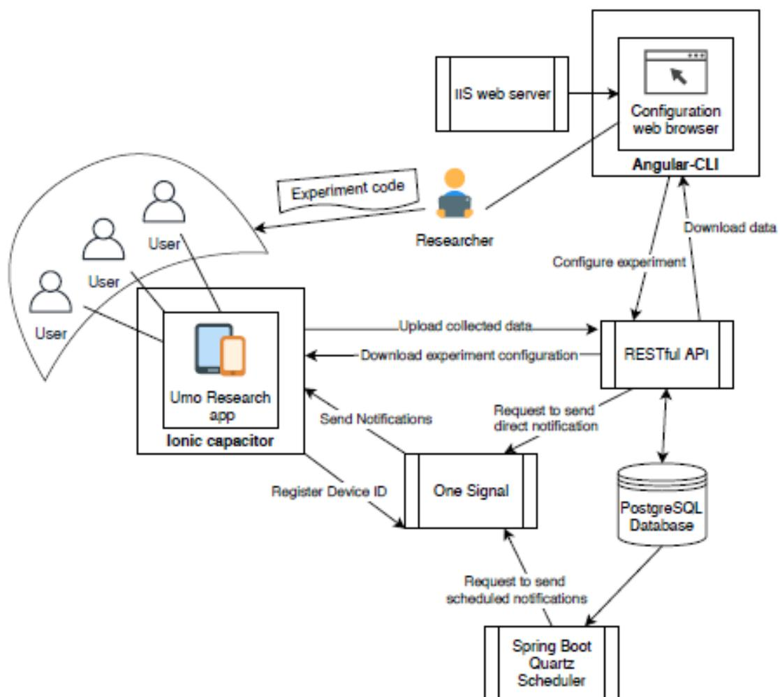
Figure 4.5. Data collection tool system architecture
