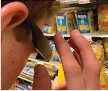
Figure 43: Reading text with the Envision smart glasses on products
