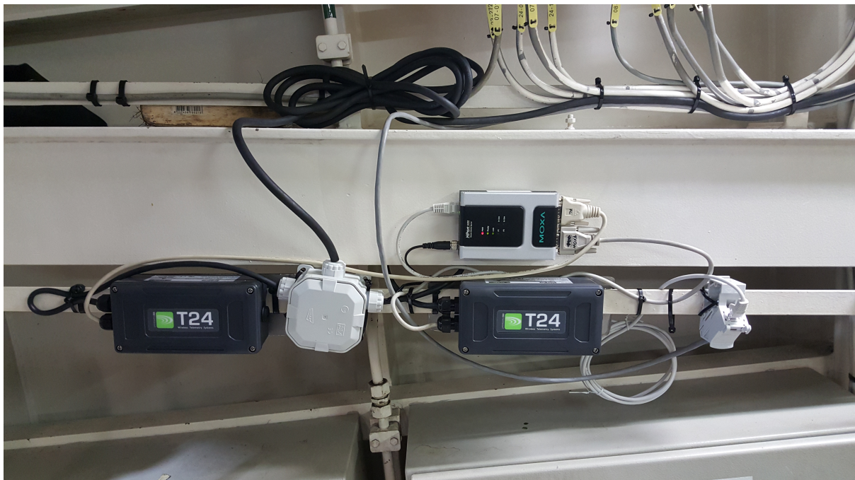
Figure 10.14: Mini Moxa N PORT series 6150 in combination with Mantracourt T24 series installed.
