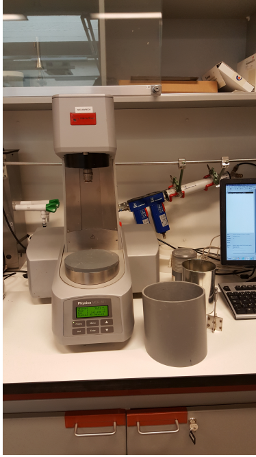
(a) The Anton Paar Rheometer used for the experiment. (b) A sample container with consolidated material.
