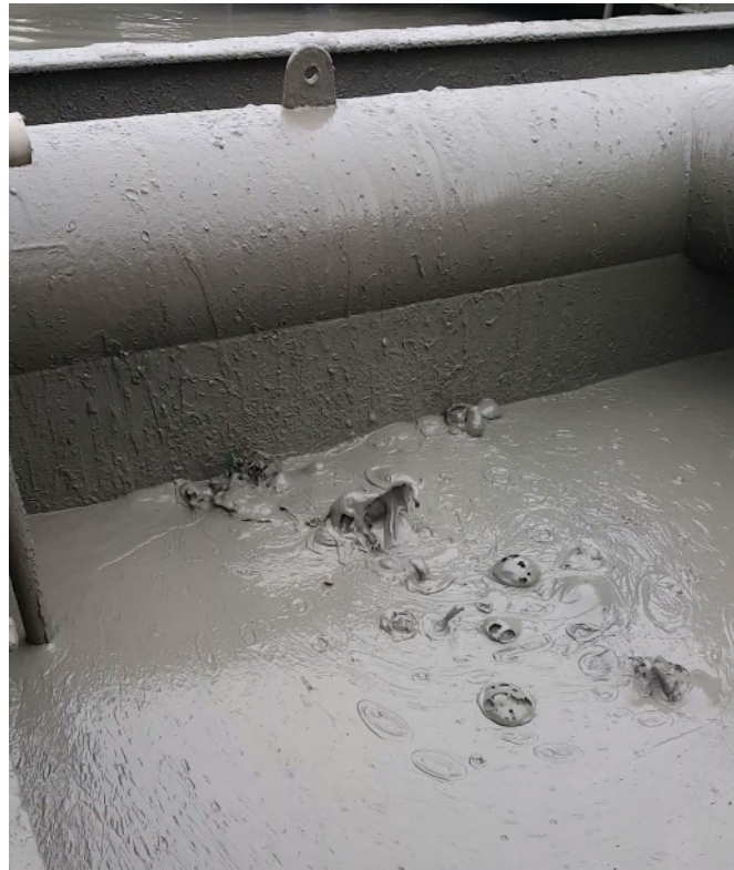
Figure 4.14: Bubbles arising from the mixture when discharged in the hopper. - ‘Pallierter’
