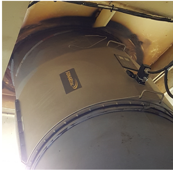
Figure 6.6: Sonartrac VF100 installed on board TSHD Pallieter.
