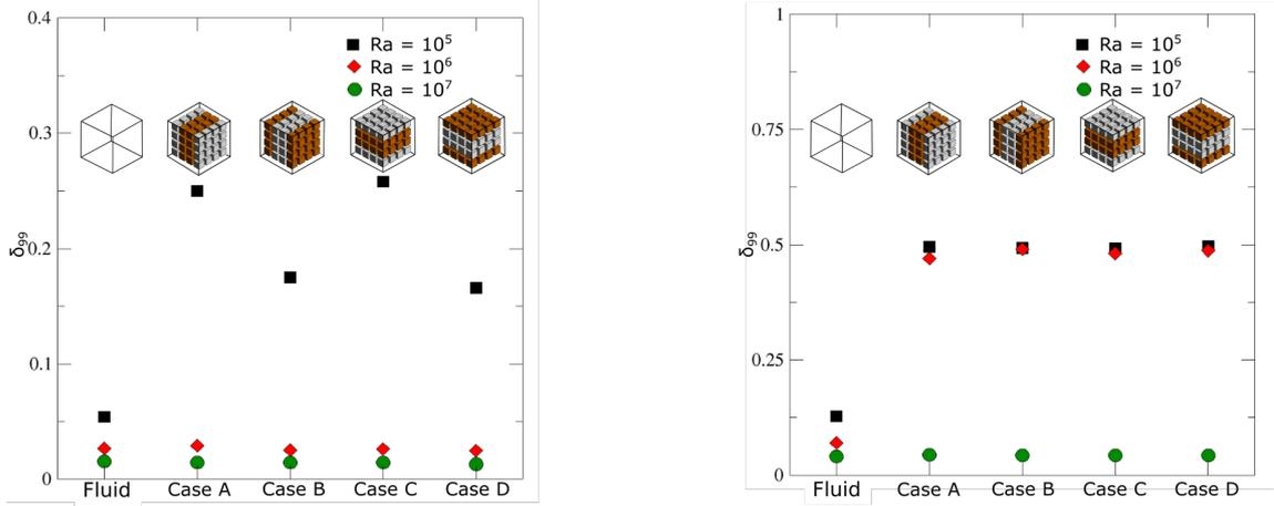
(a) The boundary layer thickness when objects are not attached to the wall at  $y/H = 0.1$
