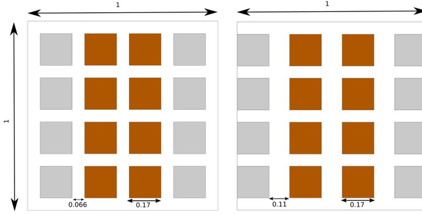
Figure 3.3: Length scales of the cases when the objects are a small distance from the wall(left) and when they are attached to the wall (right).
