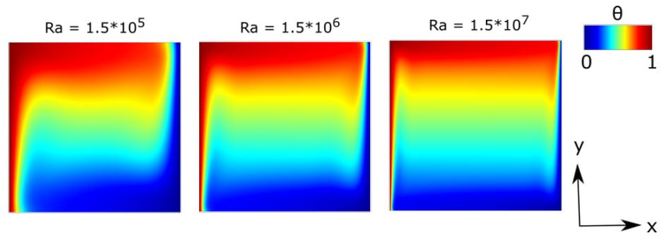
Figure 4.2: Temperature contours at  $Ra$   $10^5$ ,  $10^6$  and  $10^7$  of the only fluid case.
