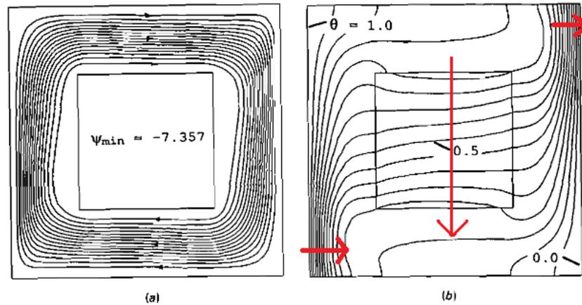
Figure 2.3: (a) Stream lines and (b) isotherms at side heated cavity of  $Ra = 10^5$  and  $\lambda^* = 0.2$ . Simulation and images performed by House[11]. The red arrows in (b) show the direction of conduction in the cavity and how conductive objects can stimulate conduction from the top to the bottom.
