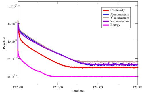
(a) Monitor of residuals of Case A with the objects not attached at  $Ra = 10^6$
