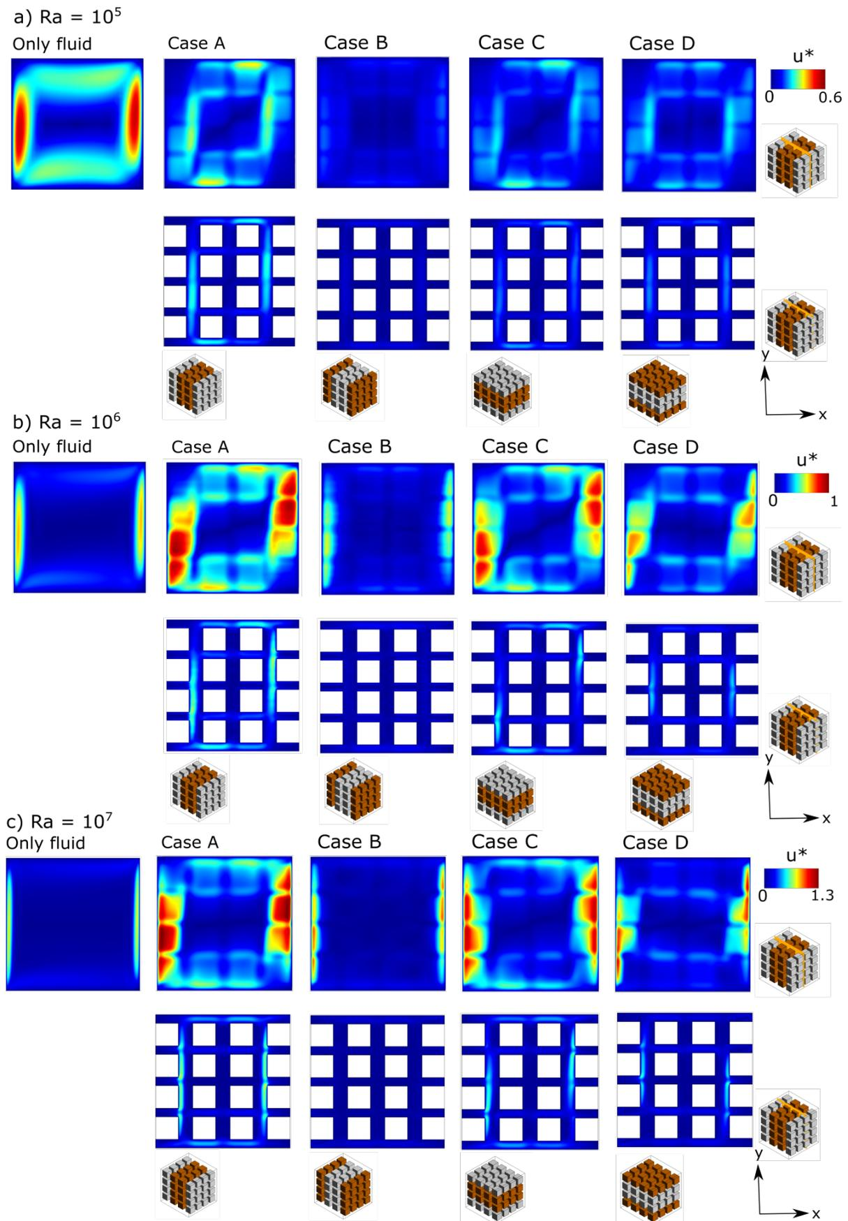
Figure 6.3: Velocity contours when objects are attached to the walls at a)  $Ra = 10^5$ , b)  $Ra = 10^6$  and c)  $Ra = 10^7$ . The contours are taken at two planes, at  $z/W = 0.5$  and  $z/W = 0.4$ .
