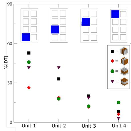
Figure 6.9: Thermal disequilibrium between objects and the fluid when the objects are attached the wall at  $Ra = 10^7$ .
