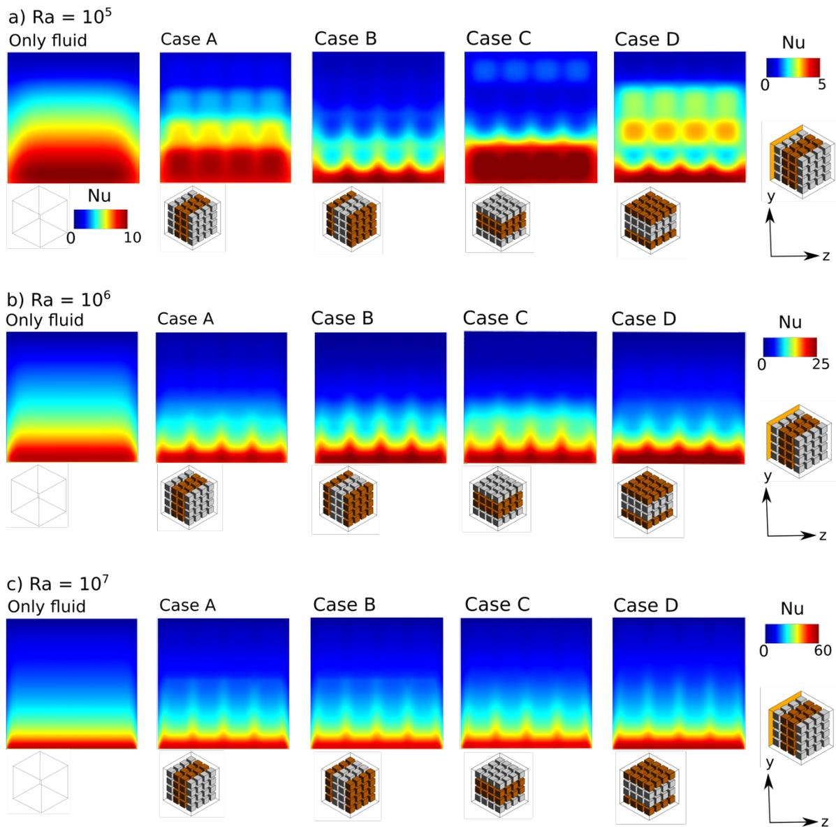
Figure 5.6: Contours of the local Nu at the hot wall when objects are not attached to the walls at a)  $Ra = 10^5$ , b)  $Ra = 10^6$  and c)  $Ra = 10^7$ .
