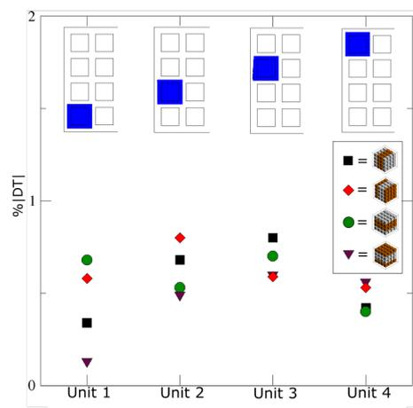
Figure 5.10: Thermal disequilibrium between objects and the fluid when the objects are not attached the wall at  $Ra = 10^7$ .
