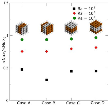
Figure 5.7: Average Nusselt number at the hot wall when objects are not attached to the wall. The  $\langle Nu \rangle$  is normalized by dividing over the  $\langle Nu \rangle$  of the only fluid case.
