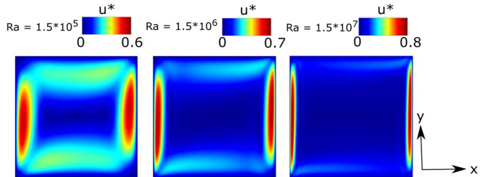
Figure 4.3: Velocity contours at  $Ra$   $10^5$ ,  $10^6$  and  $10^7$  of the only fluid case.
