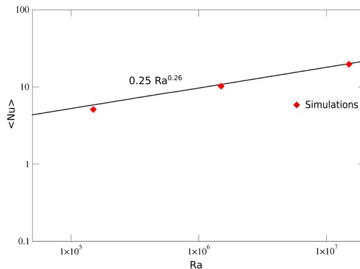
Figure 4.1: Nu number against Ra. The line represents the power law Rounaghi [26] found by doing experiments. The three diamonds are simulations of the only fluid case to validate the mesh.
