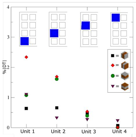
Figure 5.9: Thermal disequilibrium between objects and the fluid when the objects are not attached the wall at  $Ra = 10^6$ .
