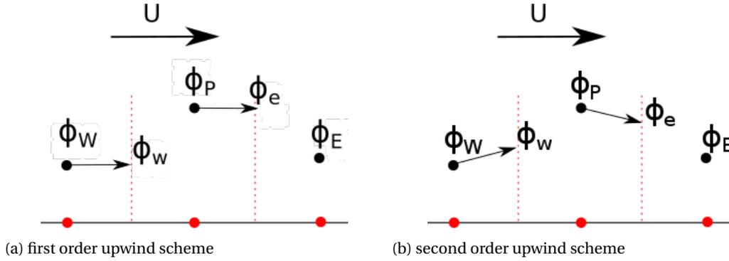
Figure 3.2: 1D schematic of the (a) first and (b) second order upwind scheme
