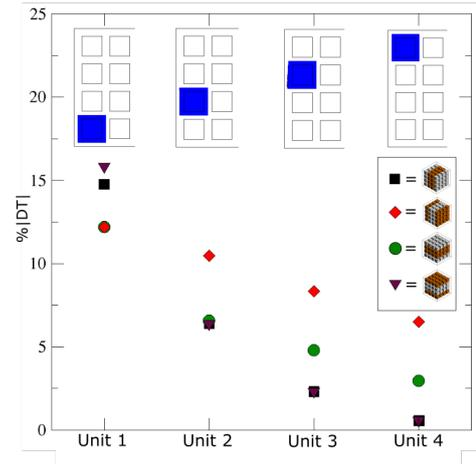
Figure 6.7: Thermal disequilibrium between objects and the fluid when the objects are attached the wall at  $Ra = 10^5$ .
