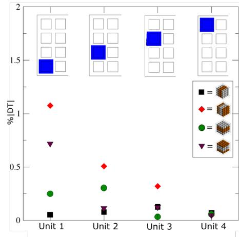
Figure 5.8: Thermal disequilibrium between objects and the fluid when the objects are not attached the wall at  $Ra = 10^5$ .
