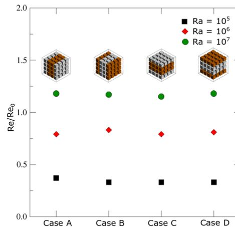
Figure 5.5: The Volume averaged RMS of Re when objects don't touch the walls. The Re is normalized by dividing to the Re of the only fluid case.
