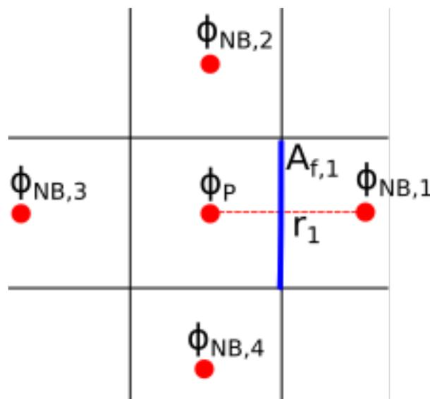
Figure 3.1: A scheme of how FVM works.
