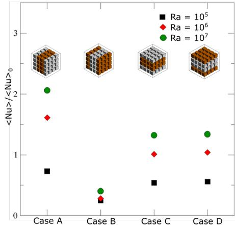
Figure 6.6: Average Nusselt number at the hot wall when objects are attached to the wall. The  $\langle Nu \rangle$  is normalized by dividing over the  $\langle Nu \rangle$  of the only fluid case.
