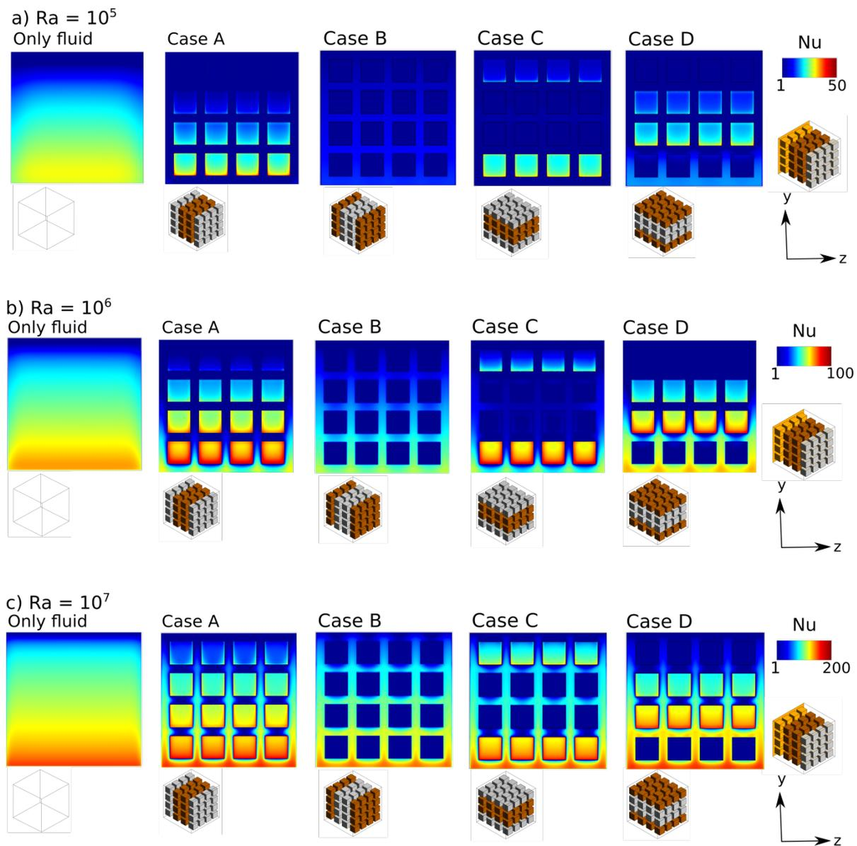
Figure 6.5: Nu contours at the hot wall and the objects attached them at a)  $Ra = 10^5$ , b)  $Ra = 10^6$  and c)  $Ra = 10^7$ .
