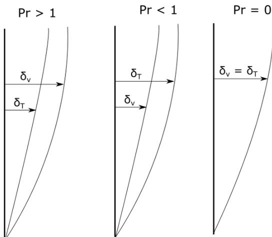
Figure 2.1: The Boundary Layer at different Pr values.
