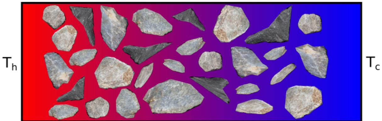
Figure 1.1: Model of the ground with a hot heat reservoir and a cold reservoir. It is filled with objects of different size and material.
