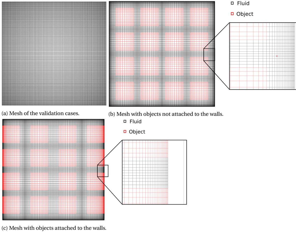
Figure 3.4: Cross-section of the three meshes used.
