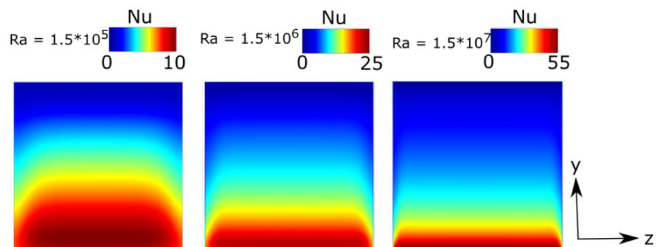
Figure 4.4: Velocity contours at  $Ra$   $10^5$ ,  $10^6$  and  $10^7$  of the only fluid case.
