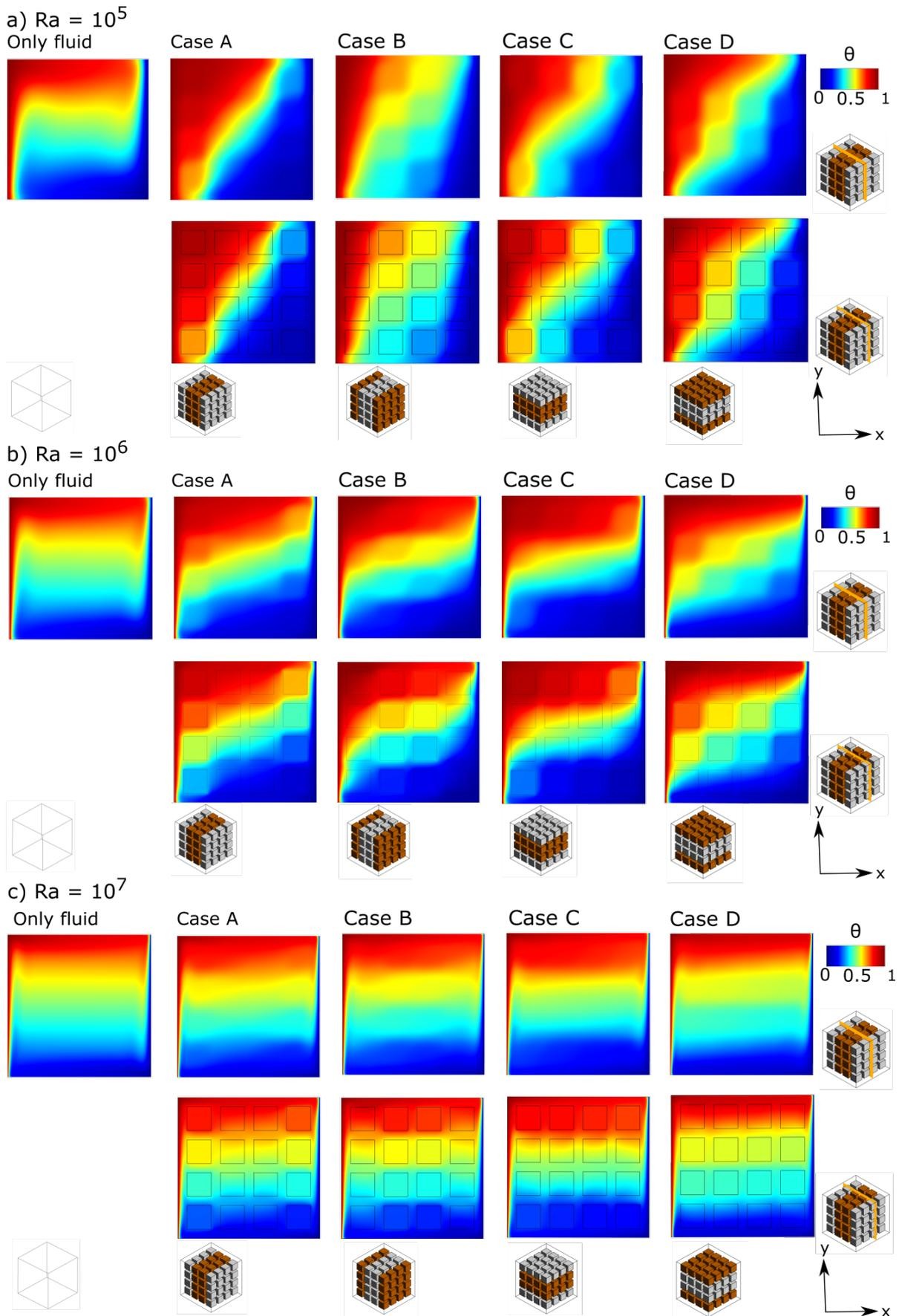
Figure 5.1: Temperature contours when objects are not attached to the walls at a)  $Ra = 10^5$ , b)  $Ra = 10^6$  and c)  $Ra = 10^7$ . The contours are taken at two planes, at  $z/W = 0.5$  and  $z/W = 0.4$ .
