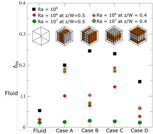
(b) The boundary layer thickness when objects are attached to the wall at  $y/H = 0.1$
