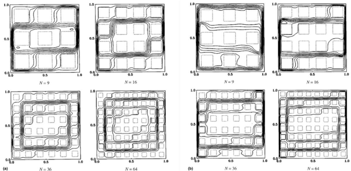
Figure 2.4: Cavity with 9, 12, 36 and 64 objects at a)  $Ra = 10^6$  and b)  $Ra = 10^7$ . Simulations and pictures done by Merrikh and Lage [15].
