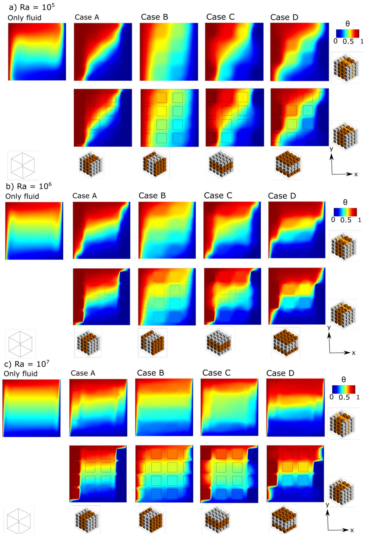
Figure 6.1: Temperature contours when objects are attached to the walls at a)  $Ra = 10^5$ , b)  $Ra = 10^6$  and c)  $Ra = 10^7$ . The contours are taken at two planes, at  $z/W = 0.5$  and  $z/W = 0.4$ .
