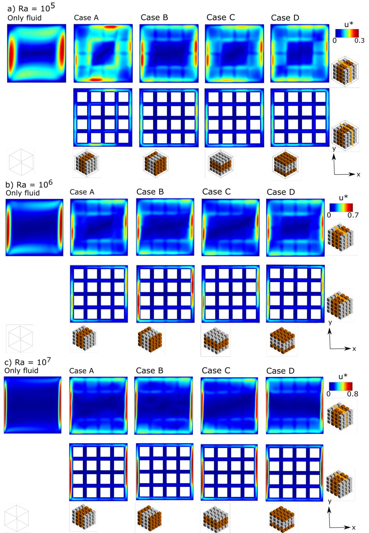
Figure 5.3: Contours of non-dimensional velocity magnitude when objects are not attached to the walls at a)  $Ra = 10^5$ , b)  $Ra = 10^6$  and c)  $Ra = 10^7$ . The contours are taken at two planes, at  $z/W = 0.5$  and  $z/W = 0.4$ .
