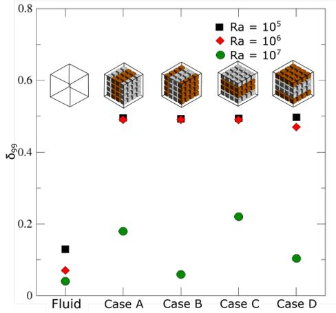
(a) The boundary layer thickness when objects are attached to the wall at  $y/H = 0.5$
