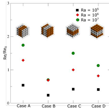
Figure 6.4: The Volume averaged RMS of Re when objects don't touch the walls. The Re is normalized by dividing to  $Re_0$  of the only fluid case.
