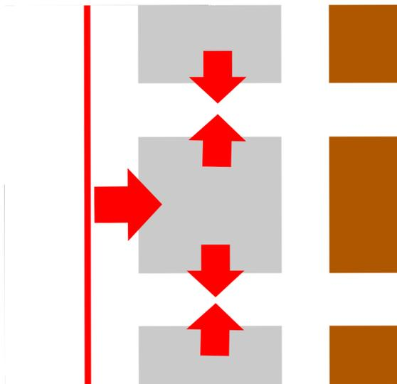
Figure 5.4: Schematic view how the conductive objects heat the fluid from the side. The heat is transferred from the wall through the conductive objects to the sides.
