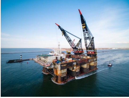
Figure 5.1: A multi-hull crane vessel [24].
