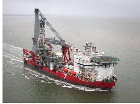
Figure 5.2: A mono-hull crane vessel [54].
