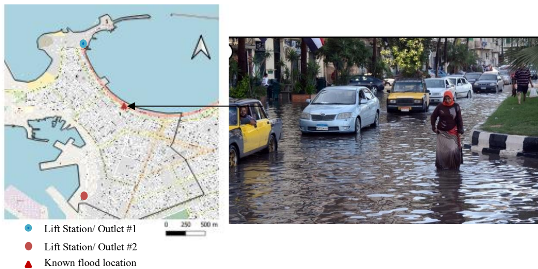
Figure 4.15 Known flooding locations in El Gomork along the Corniche Road in Alexandria. On October 25, 2015, this location experienced flooding depths ~0.15 - 0.3m.
