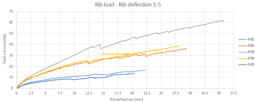
Figure 7.49: A graph showing the deflection at half of the span length for the corresponding force in the ribs.
