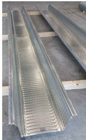
(b) One steel profiled steel deck plate lying upside down
