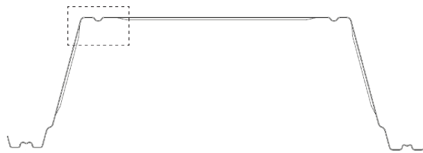
(a) The cross-section of a single plate of the COMFLOR210 steel profiled deck.
