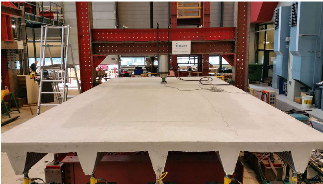
Figure 7.74: 0 mesh slab in the test set-up with the crack indicated with a marker on the top.
