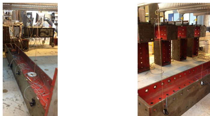
Figure 7.28: An overview of the thread LVDTs used in the lab experiments
