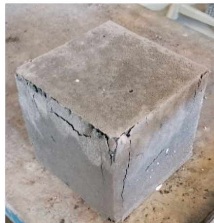
(b) A concrete cube, failed in compression
