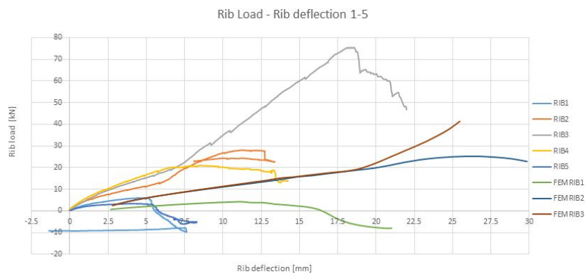
Figure 8.11: The rib load-deflection diagram found in the experiment and in the FEM model.
