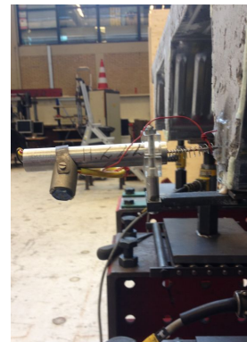
(b) An overview of an end-slip LVDT
