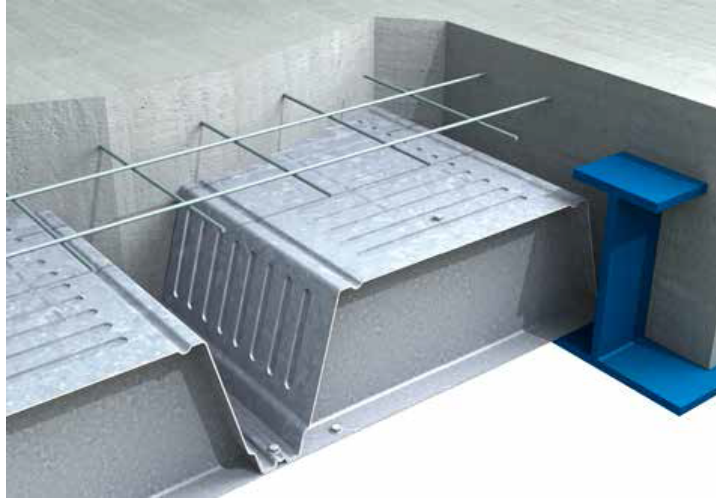
Figure 4.4: A 3D rendering of a COMFLOR210 deep composite slab
