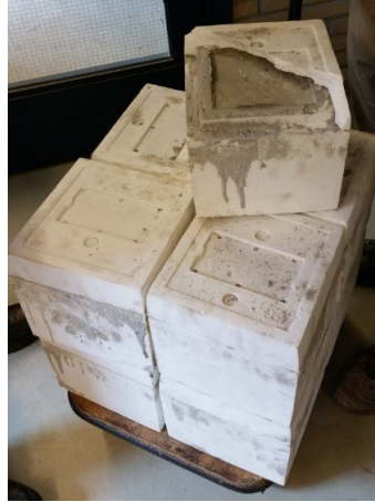
Figure F.18: One batch of concrete cubes, packed in styrofoam
