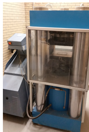
(b) Test set-up for the concrete cubes
