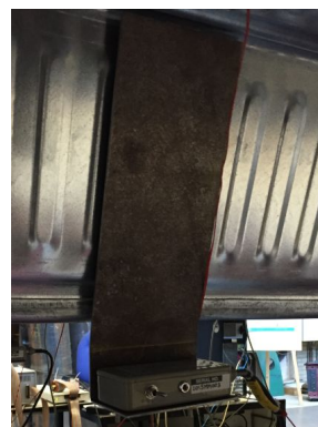
(a) The rotation gauge with metal frame
