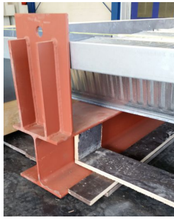
(a) The steel beams used to lift the test specimens. The upstanding stiffened steel plate is to prevent the test specimens from shifting sideways.
