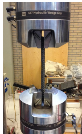
(b) Test overview tension test Ø20
