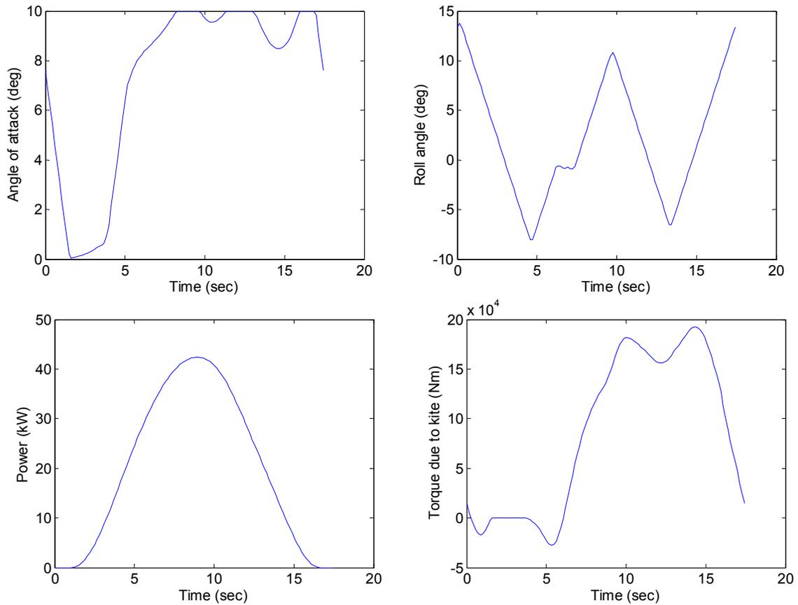
**Fig. 7 Optimal trajectories for rotating kite generator in 15 m/s wind, a) Kite angle of attack, b) Kite roll angle, c) Power extracted by generator, d) Torque of tether on lever arm.**
