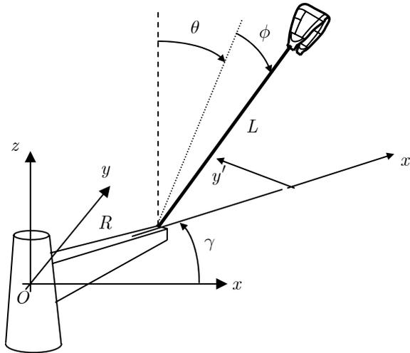
Fig. 2 Tethered kite system model.
