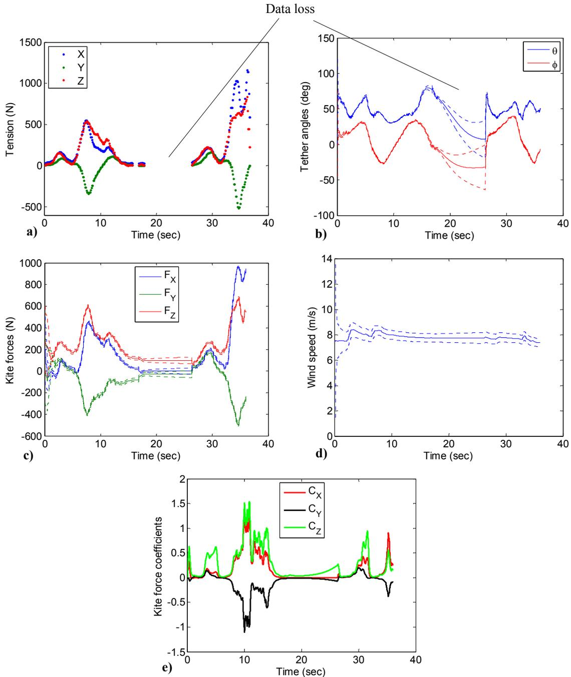
**Fig. 5 Filtered estimates of kite data, a) Tension measurements, b) Estimated tether angles and  $3\sigma$ -covariance bounds, c) Kite forces and  $3\sigma$ -covariance bounds, d) Wind speed and  $3\sigma$ -covariance bounds, e) Force coefficients.**
