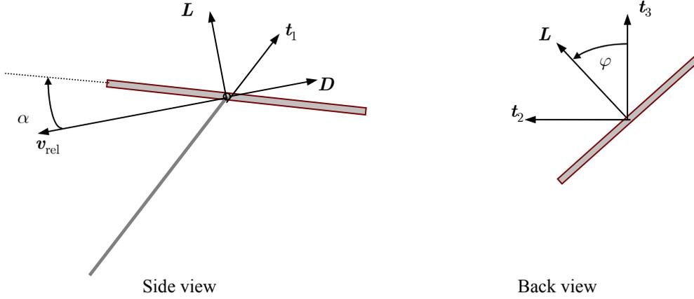
**Fig. 4 Lift and drag forces on kite.**
