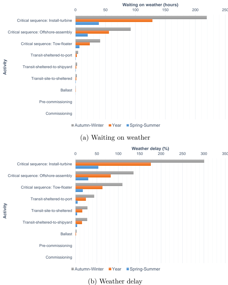
Figure 3.10: Waiting on weather and weather delay of installation activities of the spar buoy installation with crane barge for the three examined time periods.
