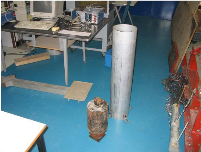
Figure 6.6 Guidance tube and drop mass with spring assembly
