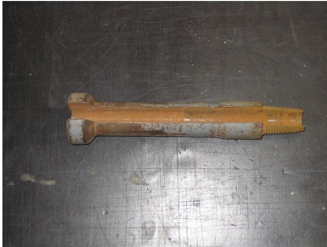
Figure 6.14 Side guide of cable at the pile head
