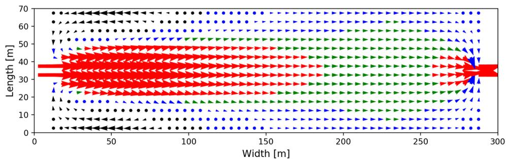
Figure 3.2: Case B: W = 70 m; L = 280 m; W/L-ratio = 1/4. Flow pattern shown by depth average flow velocity in 2DH. Green:  $\approx 2DV$  flow velocity. Red:  $> 2DV$  flow velocity. Blue:  $< 2DV$  flow velocity. Black: no flow or  $< 0$  m/s.
