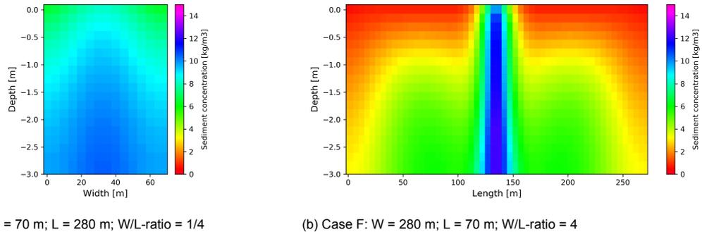
Figure 3.6: Sediment dispersion over the middle cross-sections for two basins
