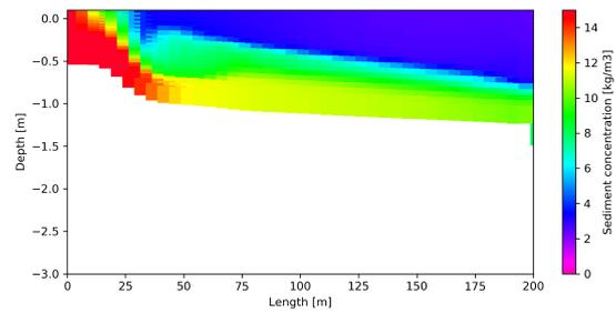
(b) Spread plot case B: wind = 10 m/s
