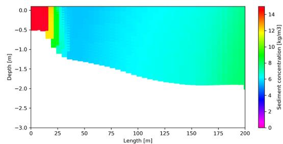
(b) Spread plot case B: wind = 25 m/s
