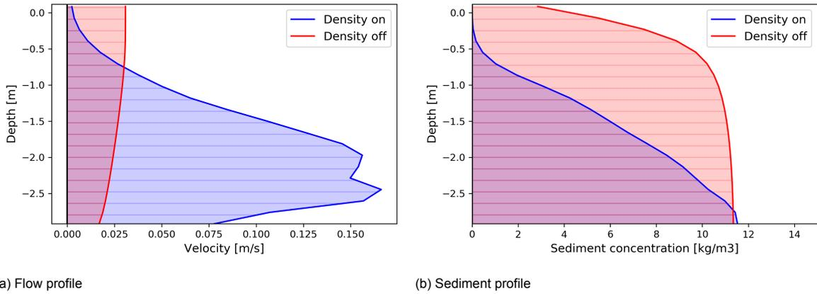
Figure 3.13: Density driven currents in the middle grid cell of the basin. Left: flow profile. Right: sediment concentration profile.
