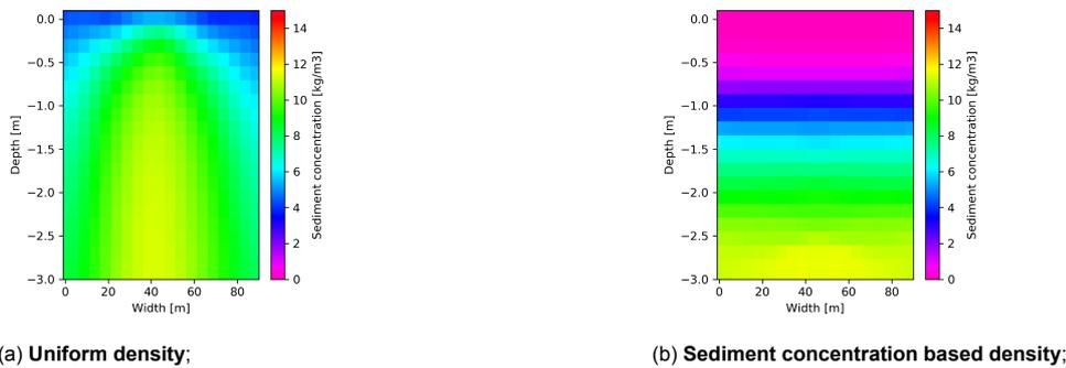
Figure 3.11: Cross-section of sediment concentration over the width of the basin (at  $x = 1/2 L$ ).
