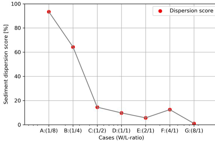
Figure 3.7: Width uniform sediment dispersion score. Horizontal axis: W/L-ratio (logarithmic scale). Vertical axis: uniformity score in percentages.
