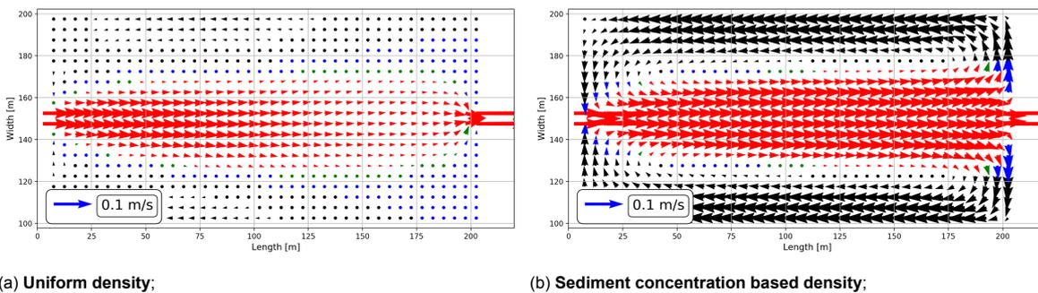
Figure 3.12: Flow pattern for the base case (Case C). Comparison to show the influence of density driven currents.
