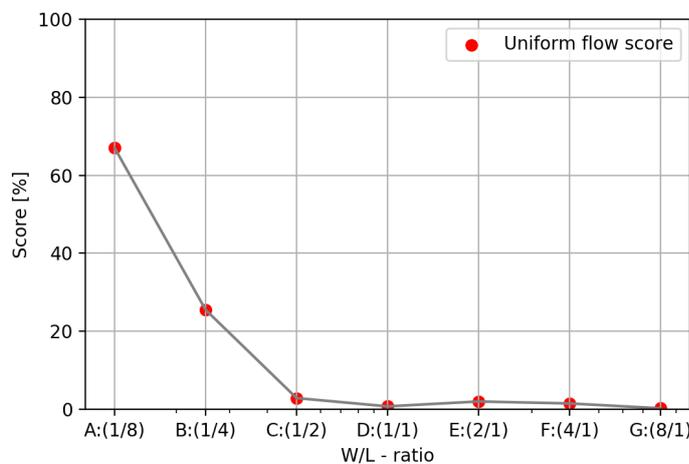
Figure 3.4: Width uniform flow conditions score. Horizontal axis: W/L-ratio (logarithmic scale). Vertical axis: uniformity score in percentages.
