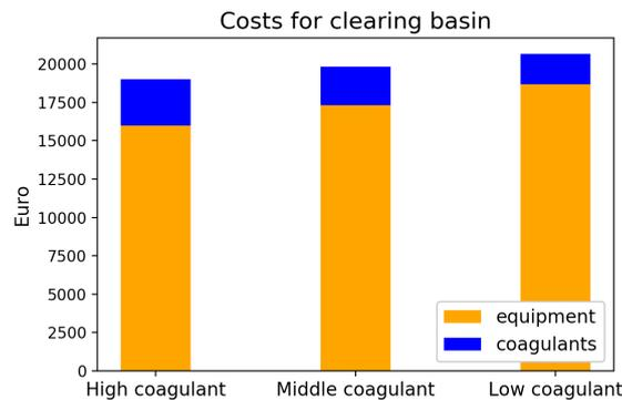
Figure 5.1: Costs for clearing basin at the Grensmaas. This visualization shows the (increase in) equipment costs is much larger than the (decrease in) costs for coagulants.
