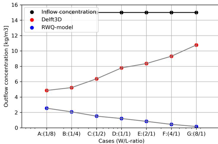
Figure 3.8: Outflow concentration for the geometry cases, width uniform conditions scenario. Red: Delft3D. Blue: RWQ model. Horizontal axes: W/L-ratio per case. Vertical axes: Outflow concentration.
