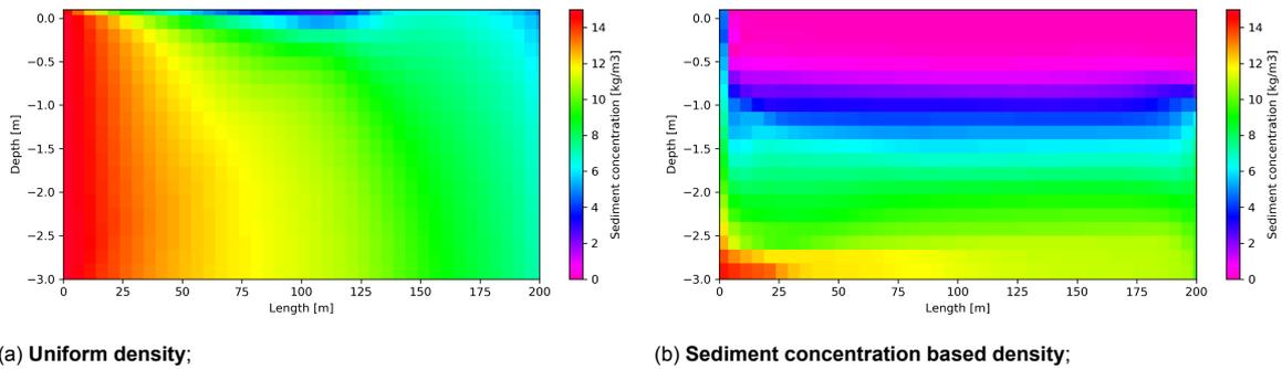
Figure 3.10: Cross-section of sediment concentration over the length of the basin (at  $y = 1/2 W$ ).
