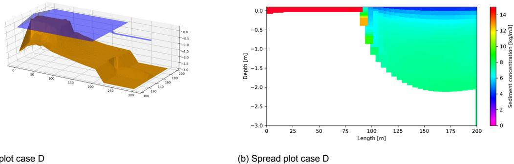
Figure 4.4: Filling behaviour case D
