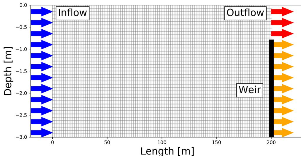
Figure 2.1: Grid of the RWQ model in 2DV. Vertical axes: depth [m]. Horizontal axes: length [m]. Blue arrows: inflow. Orange and red arrows: outflow. Red arrows: upper 25 % of the water column determining the outflow concentration. The grey grid shows the computational area.
