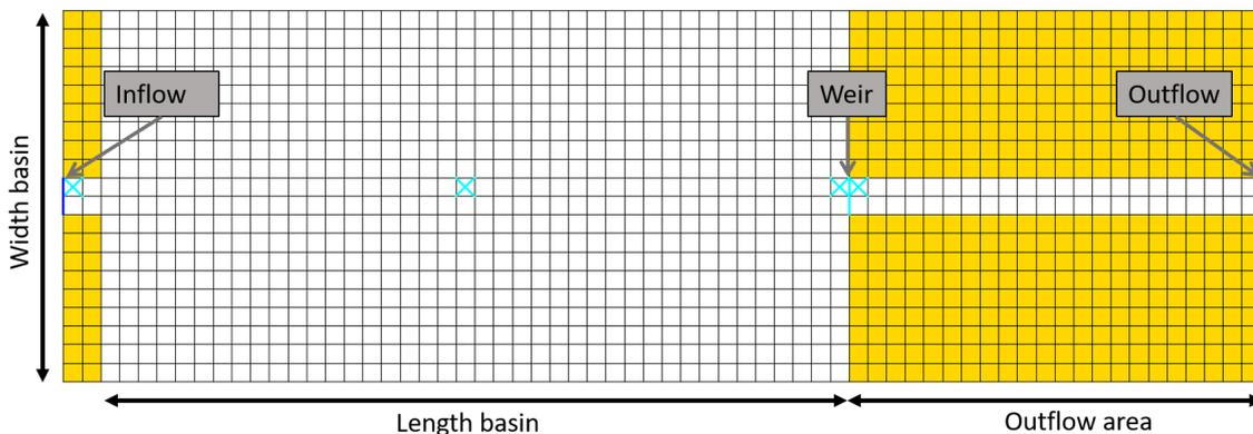
Figure 2.2: Presentation of Delft3D grid. This figure (from Delft3D) presents the grid of the base case with important elements accented. White grid cells: computational area. Yellow grid cells: dry points (used to mark the edge of the basin and inactive cells).
