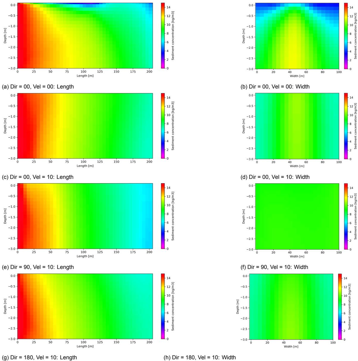
Figure 3.16: Additional mixing due to wind from all directions.
