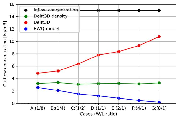
Figure 3.15: Outflow concentration for different basin geometries (W/L-ratio). Density differences on (Delft3D, green), density differences off (Delft3D, red) and RWQ-model (blue).
