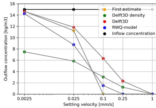
Figure 3.1: Comparison of outflow concentrations for base case with changing settling velocity compared when calculated with the simple sum.
