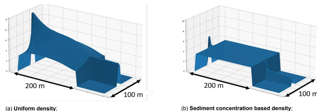
Figure 3.9: Average sediment concentration over the water column through the basin.
