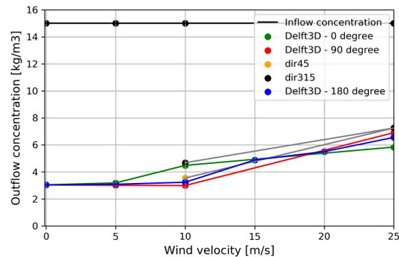
Figure 3.20: Outflow concentration for the scenario with density and wind combined. The dots are results from cases. The lines are interpolations between the results.
