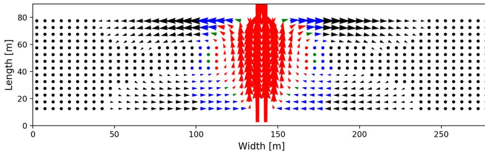
Figure 3.3: Case F: W = 280 m; L = 70 m; W/L-ratio = 4. Flow pattern shown by depth average flow velocity in 2DH. Green:  $\approx 2DH$  flow velocity. Red:  $>2DV$  flow velocity. Blue:  $<2DV$  flow velocity. Black: no flow or  $<0$  m/s.
