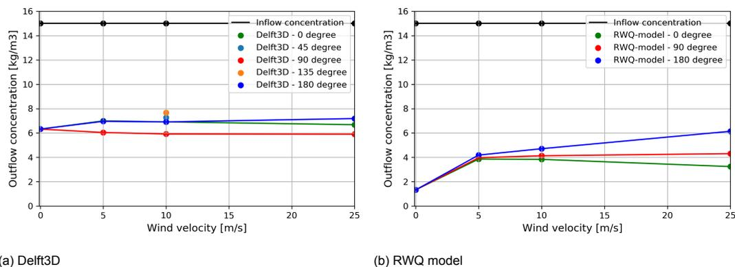
Figure 3.18: Outflow concentration affected by wind.
