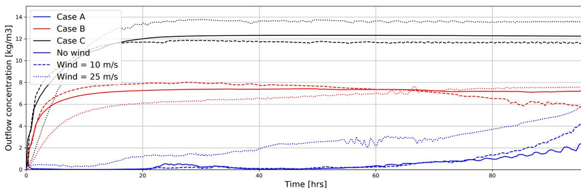
Figure B.1: Outflow concentration over time for different wind velocities
