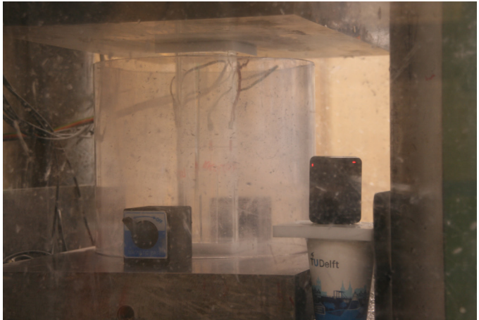
Figure 100: the tube for catching shrapnel was held in place by magnets and most experiments could be filmed
