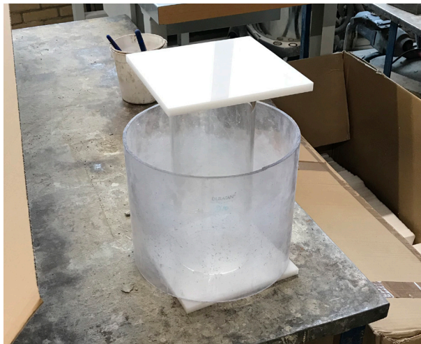
Figure 108: shrapnel blocking tube was placed over the samples to avoid glass particles causing potential harm
