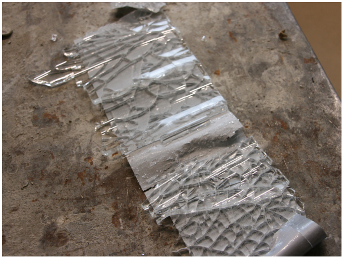
Figure 113: shattering pattern of hardened samples, held together by duct tape
