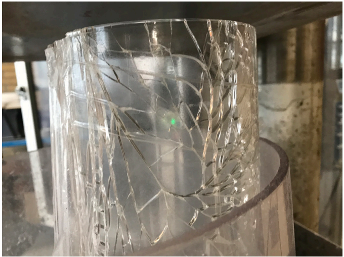
Figure 112: the hardened samples would display these kinds of shattering patterns
