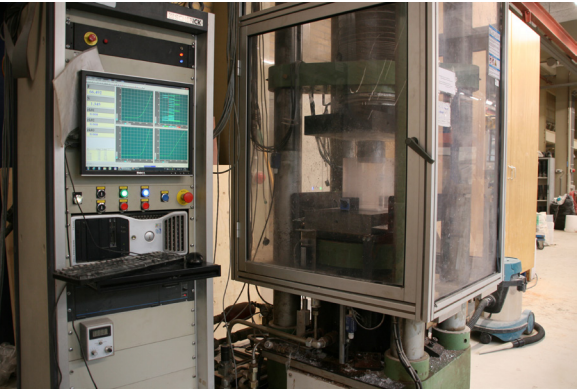
Figure 56: the Toni-bank used for the compressive tests
