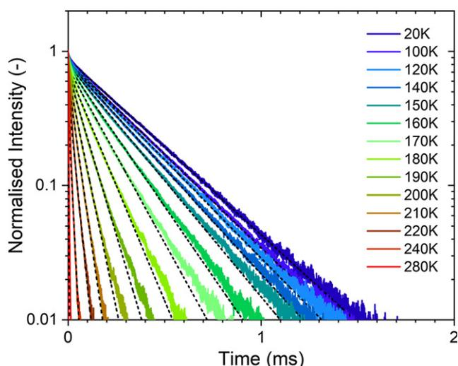
**Figure 4.** Normalised luminescence lifetime curves of 5d–4f emission  $R_{20}$  plotted at various temperatures. The dashed lines represent the single exponential fits based on our rate equations from which  $W_{21}(T)$  values were obtained.
