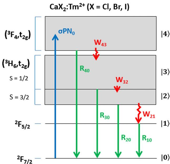
**Figure 3.** Schematic energy level diagram for  $\text{CaX}_2:\text{Tm}^{2+}$  upon exciting into the ( ${}^3\text{F}_4, \text{t}_{2g}$ ) levels (blue arrow). At 20 K up to four distinct  $\text{Tm}^{2+}$  emissions are observed. These radiative transitions are indicated by the green straight arrows  $R_{ij}$ , while non-radiative quenching transitions  $W_{ij}$  are indicated by the red curly arrows. Here, index  $i$  refers to starting level and  $j$  the closing level.
