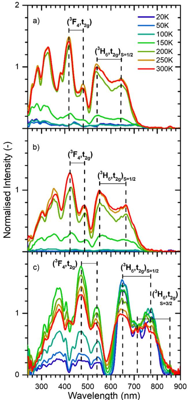
**Figure 1.** Normalised excitation spectra of: (a)  $\text{CaCl}_2:\text{Tm}^{2+}$ , (b)  $\text{CaBr}_2:\text{Tm}^{2+}$  and (c)  $\text{CaI}_2:\text{Tm}^{2+}$  as acquired on the  $\text{Tm}^{2+} \ ^2\text{F}_{5/2} \rightarrow \ ^2\text{F}_{7/2}$  4f–4f emission at 1140 nm and for different temperatures. The spectra are normalised on the LS  $(^3\text{H}_6, \text{t}_{2g})_{S=1/2}$  band at 300 K.
