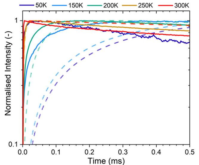
**Figure 8.** Normalised luminescence lifetime curves of  $4f-4f$  emission  $R_{10}$  plotted at various temperatures, clearly displaying a risetime phenomenon. The solid curves represent experimental data, whereas the dashed transparent curves are plots based on our combined quenching model.
