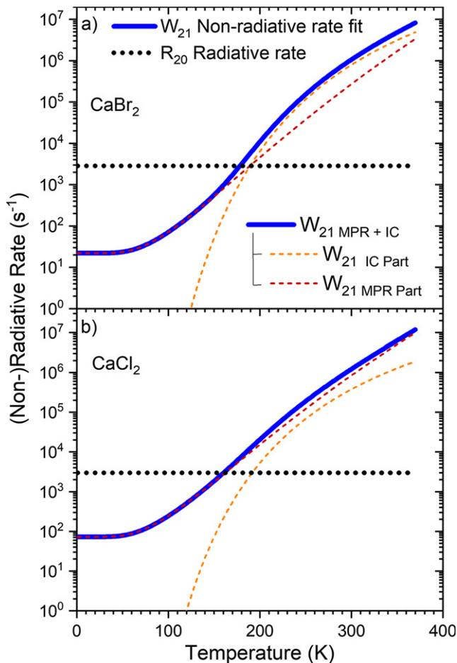
**Figure 7.** The obtained  $W_{21}$  parameters of (a)  $\text{CaCl}_2:\text{Tm}^{2+}$  and (b)  $\text{CaBr}_2:\text{Tm}^{2+}$  plotted in blue and versus temperature. The dark red and orange dashed lines respectively reveal the MPR and IC constituents, while the dotted black line shows the  $R_{20}$  radiative rate.
