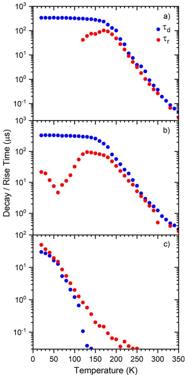
**Figure 9.** Temperature dependence of the lifetime ( $\tau_d$ ) related to the 5d–4f ( ${}^3\text{H}_6, t_{2g}$ ) HS emission and risetime ( $\tau_r$ ) of the 4f–4f emission in: (a)  $\text{CaCl}_2:\text{Tm}^{2+}$ , (b)  $\text{CaBr}_2:\text{Tm}^{2+}$  and (c)  $\text{CaI}_2:\text{Tm}^{2+}$ . The emissions were monitored after excitation into the ( ${}^3\text{H}_6, t_{2g}$ ) LS levels.
