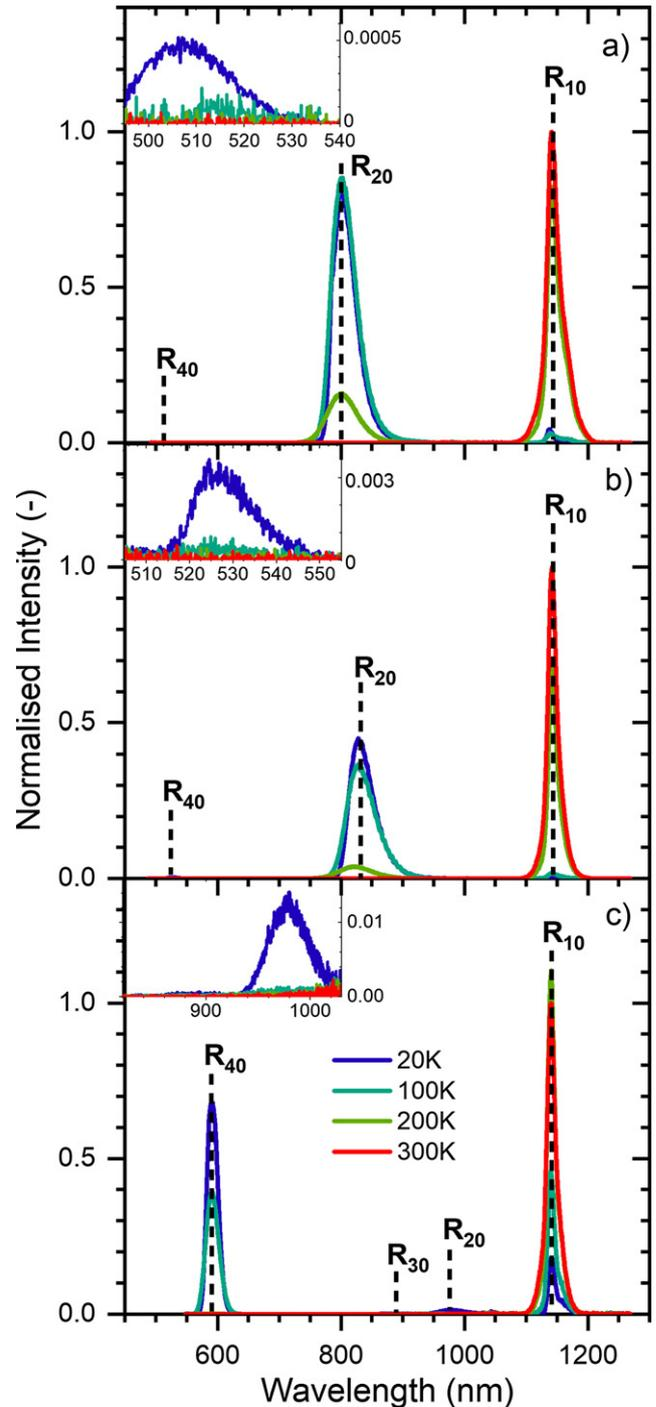
**Figure 2.** Normalised emission spectra of: (a)  $CaCl_2:Tm^{2+}$ , (b)  $CaBr_2:Tm^{2+}$  and (c)  $CaI_2:Tm^{2+}$  at different temperatures and normalised on the  $Tm^{2+} \ ^2F_{5/2} \rightarrow ^2F_{7/2}$  emission at  $300\text{ K}$ . Photoexcitation occurred within the  $(^3F_4, t_{2g})$  levels at respectively  $480\text{ nm}$ ,  $490\text{ nm}$  and  $535\text{ nm}$ .
