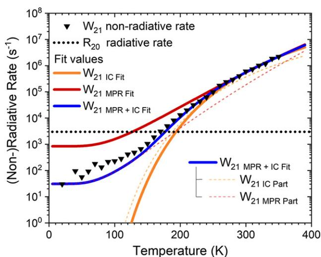
**Figure 5.** The obtained  $W_{21}$  values from figure 4 plotted as black triangular points versus temperature. The fit based on purely MPR is shown in solid dark red, whereas that of IC is displayed in solid orange. The fit of the combined quenching (MPR + IC) is illustrated in blue with constituents MPR and IC respectively portrayed in dashed red and orange. The dotted black line shows the  $R_{20}$  radiative rate.
