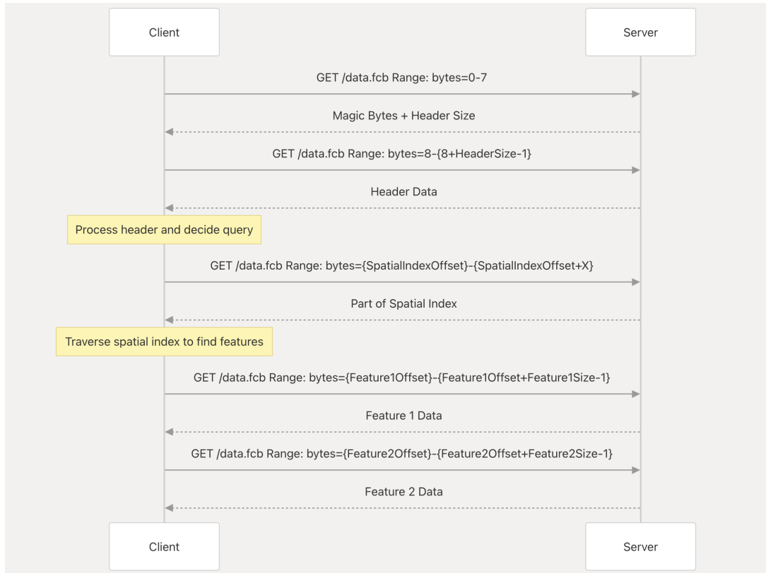
Figure 4.8.: HTTP Range Request workflow in FlatCityBuf showing the sequential process of header retrieval, index navigation, and selective feature retrieval. The client makes targeted requests for specific byte ranges rather than downloading the entire dataset.
