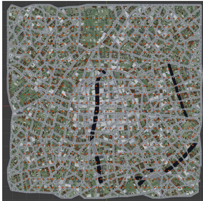
Figure 4.4.: Camera location planning. Every orange dot is a location of one camera in the extent of the synthetic city.
