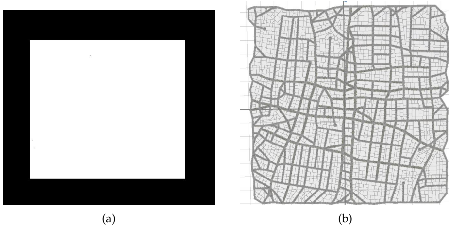
Figure 4.1.: (a) boolean control map (b) Street network with organic pattern for primary streets and raster for secondary streets
