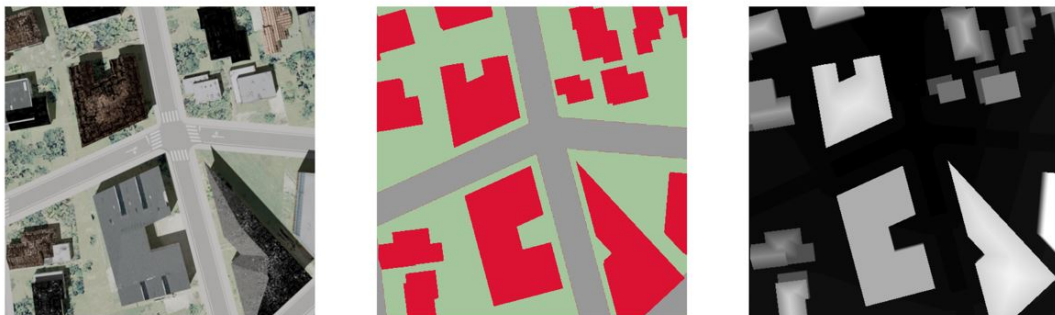
Figure 5.1.: Sample Image from the default settings of CityEngine. Left: RGB image; center: segmented image; Right depth image. Red = Building, Gray = Road and Green = Other.
