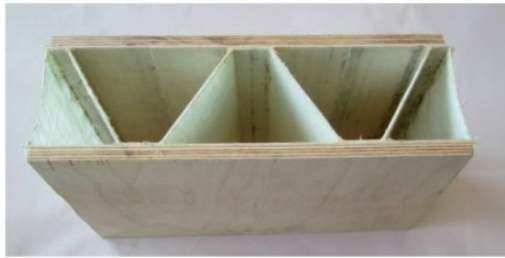
Figure 5. Sandwich panel with plywood face sheets and GF/PP core (PW_GF).
