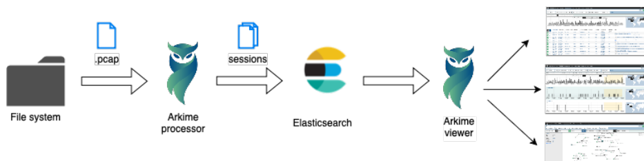
Figure 5.1: PCAP processing pipeline
