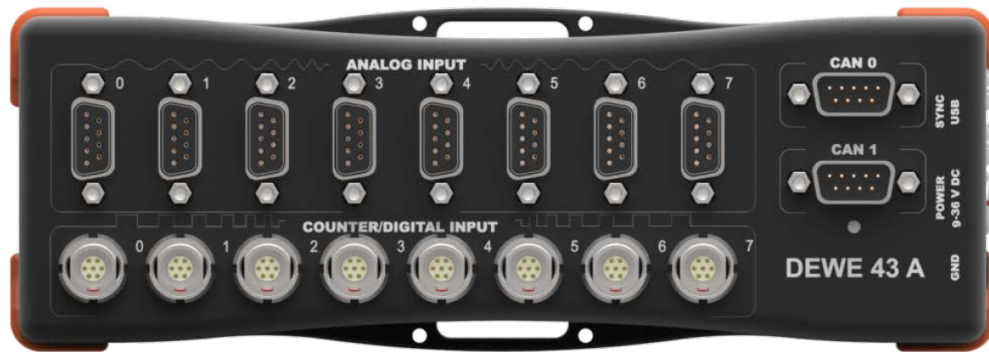
FIGURE 80: Channels of DEWE-43 board
