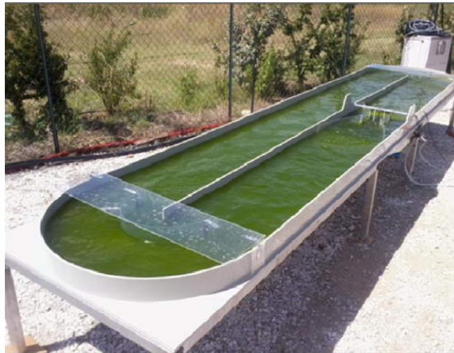
Figure 4 Picture of a 5 m 2 standard raceway reactor for microalgae taken from the paper of Chiamonti et al. (2012) 44 .
