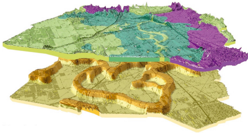
Figure 4.4: Soil types in the cover layer and the underlying aquifer. Purple: peat, tints of green: two types of clay, brown: paleochannels. The northern side of the polder is directed to the left. [105]
