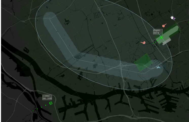
Fig. 8 Geofence activated not to protect an area from UAV operations but to vector the selected UAV behind the landing manned aircraft.
