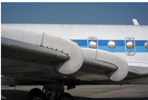
Figure 1.4: Wing fences on the wing of a Sud Aviation SE210 Caravelle [2]
