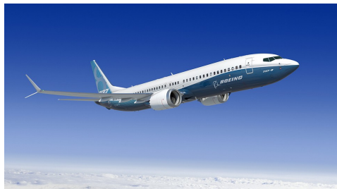
Figure 1.12: Split type winglet on a b737-MAX ©Boeing
