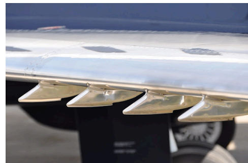
Figure 1.7: Detail view of vortilons [4]
