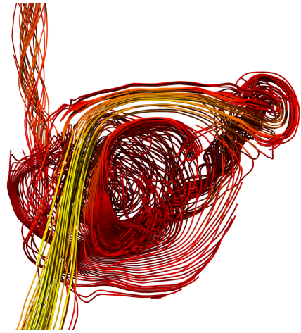
Figure 7.4: Streamlines of the measured flow after our method was applied. All visualization parameters (number of lines, seeding position, cutting plane and camera parameters) are equal to those in Figure 7.3. Note that the flow features are preserved while more streamlines are visible due to the lack of divergence and flow not leaving the segmentation.
