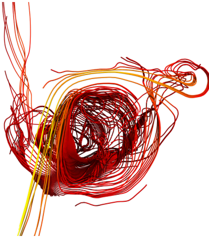
Figure 7.3: Streamlines of the measured flow before our method was applied. All visualization parameters (number of lines, seeding position and cutting plane) are equal to those in Figure 7.4. Note the presence of a vortex in the top-right corner and the helical flow present in the top-left corner and from the centre towards the top-right corner.
