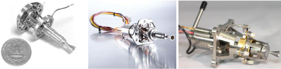
(a) Bradford ECAPS HPGP 100 mN thruster, (b) Bradford ECAPS HPGP 1 N thruster, (c) Aerojet Rocketdyne GR1 thruster, cropped from [86].
