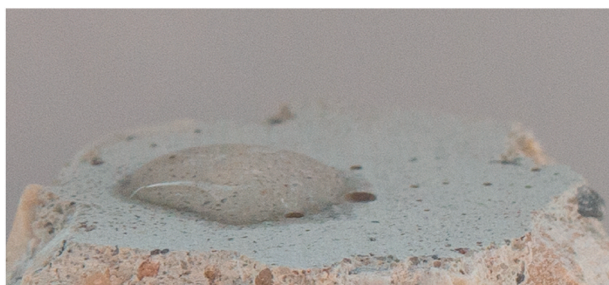
Fig. 14. Contrary to the samples where a surface retarder was used, which absorbed water almost immediately, the ones without surface retarder showed a significant delay in water absorption, causing distinct welling of water applied to their surface. This effect was still visible on this sample 3 months after casting.
