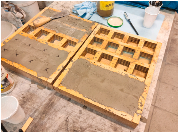
Fig. 1. The plywood moulds used for the creation of the concrete samples (left).
