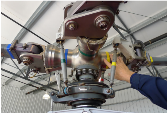
(a) The big bolt is the lead-lag hinge
