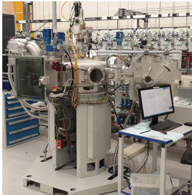
**Figure 5. Sputtering setup for IO:H deposition**
