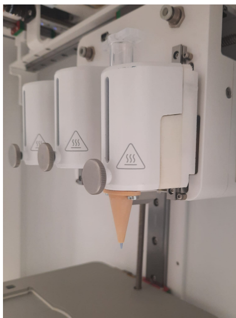
Figure 2.8: UV nozzle protector installed on a pneumatic printhead for the BIO X (CellInk) Bioprinter
