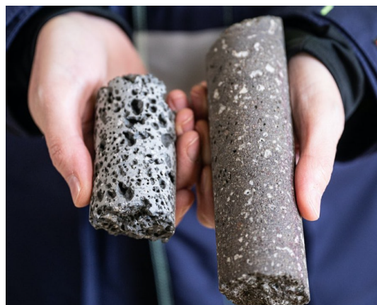
Figure 1.2: Picture of cores with CO 2 mineralized in their pores. Source: CarbFix.
