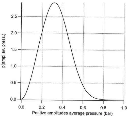
Fig. 15: Weibull probability distribution of amplitudes of average pressure, 4 transducers in middle row
