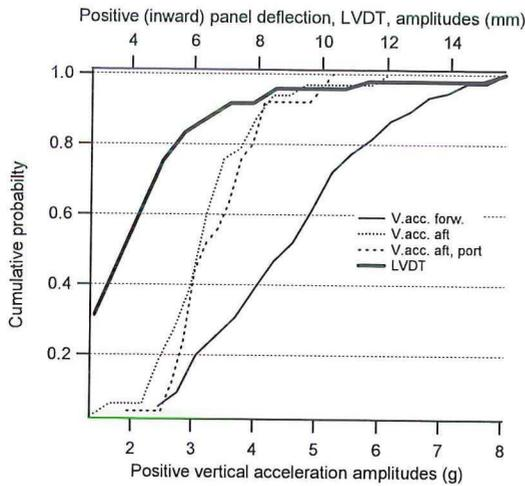
Fig. 11: Cumulative probability of amplitudes of vertical accelerations and panel deflections.
