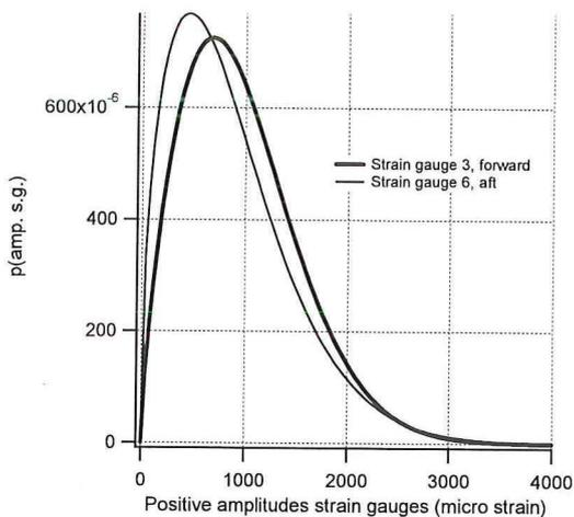
Fig. 16: Weibull probability distribution of amplitudes of strain gauge 3 forward, and 6 aft.
