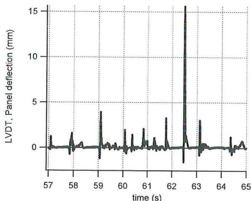
Fig. 8: Panel deflection, LVDT (mm)
