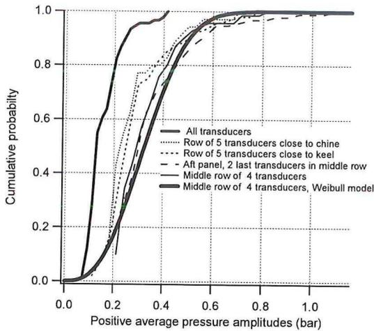
Fig. 12: Cumulative probability of amplitudes of average pressures
