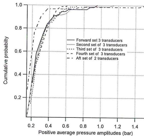
Fig. 13: Cumulative probability of amplitudes of average pressures
