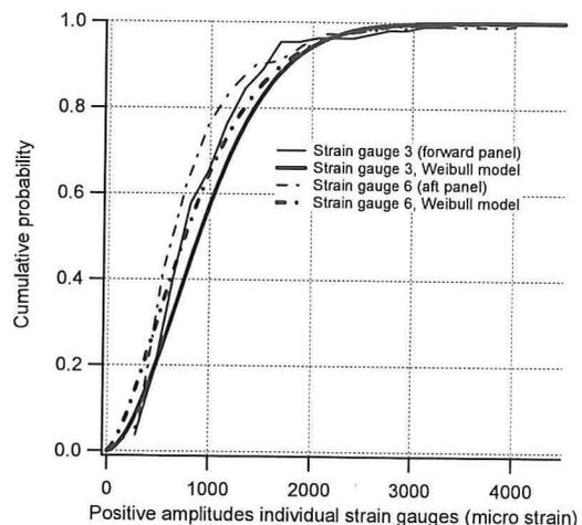
Fig. 14: Cumulative probability of amplitudes for strain gauges
