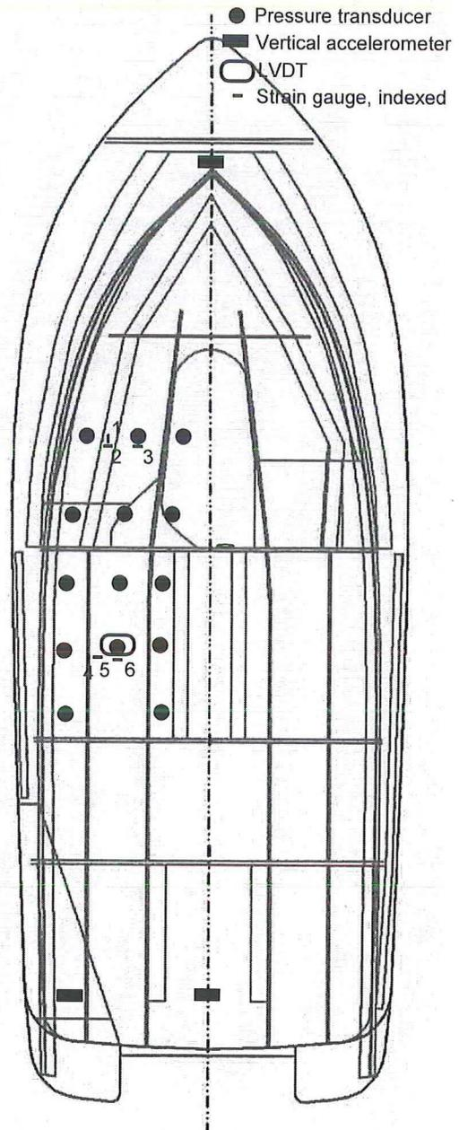
Fig. 4: Instrumentation
