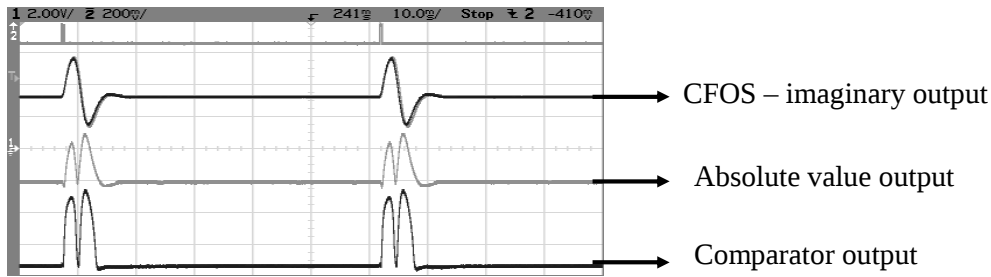
Figure 7.26: Measured output transient of the filter, the absolute and the comparator circuits
