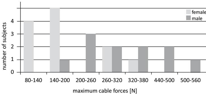
**Figure 2–3.** Male subjects attained significantly higher forces than female subjects ( $t(22)=9.89$ ,  $p < 0.001$ ). Subjects created cable forces of  $257 \pm 124$  N (mean  $\pm$  standard deviation). The maximum attained forces range from 87 to 360 N ( $188 \pm 87$  N) and 199 to 538 N ( $332 \pm 117$  N) for female and male subjects, respectively.
