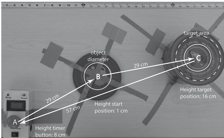
**Figure 3–5.** Visualization of one trial. The subject hits the self-timer button A to start the time measurement, moves 29 cm to grasp the object at the lower area B, then moves the object 29 cm to the higher target area C. After releasing the object, the subject needs to hit the self-timer to stop the time measurement.
