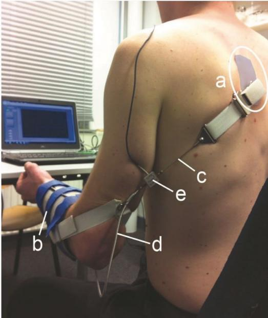
**Figure 5–1.** The Anchor System (a) is connected to a thermoplastic shell (b) via a Bowden cable (c) running inside a cable housing (d). There is a force sensor (e) in the middle of the Bowden cable to measure the cable operation forces. The original color (transparent) of the Anchor System was edited to clearly show its dimensions in the figure.
