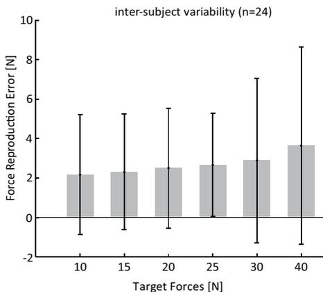
**Figure 4–7.** The force reproduction error for the 'no cable excursion' trials shows no significant differences between the tested conditions of target forces between 10 and 40 N. The bars indicate the group's average and the whiskers the standard deviation.
