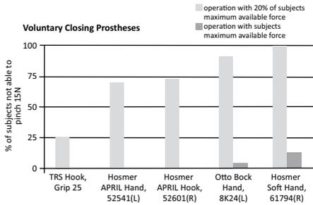
**Figure 2-4.** Pinching 15 N repetitively with five voluntary closing prostheses fatigue-free is impossible for 26 to 100% of prosthesis users. Fatigue-free operation is considered at 20% of users’ maximum cable force (38) and is desired for ADL. Cable forces required to pinch 15 N with five voluntary closing prostheses vary between 33 and 131 N (32). The maximum strength of 13% of prosthesis users is insufficient to pinch 15 N with the Hosmer Soft Hand.
