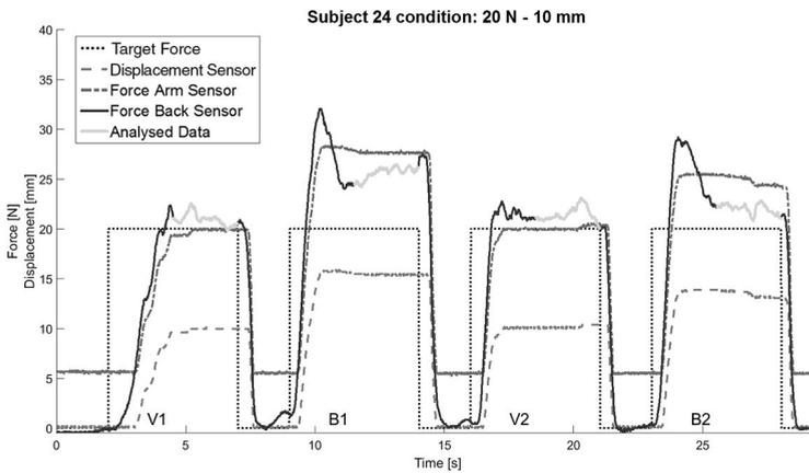
**Figure 4-6.** The raw data of the first 30 seconds of a typical trial, condition 20 N – 10 mm, represents the target force of 20 N, the approximate 10 mm cable excursion measured by the displacement sensor and the two cable forces measured at the arm ( $F_{arm}$ ) and the back ( $F_{back}$ ) of the subject. Visual blocks (V1, V2) are alternating with blind blocks (B1, B2). The last 2,5 seconds of each block were used for analysis.
