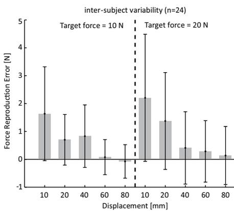
**Figure 4–9.** The force reproduction error decreases with increasing cable excursion for the ‘cable excursion’ trials for both target forces of 10 and 20 N. The force reproduction error does not differ between force levels. The zero line indicates when the target force is met. A negative force reproduction error indicates a lower reproduced force than target force. The bars indicate the group’s average and the whiskers the standard deviation.
