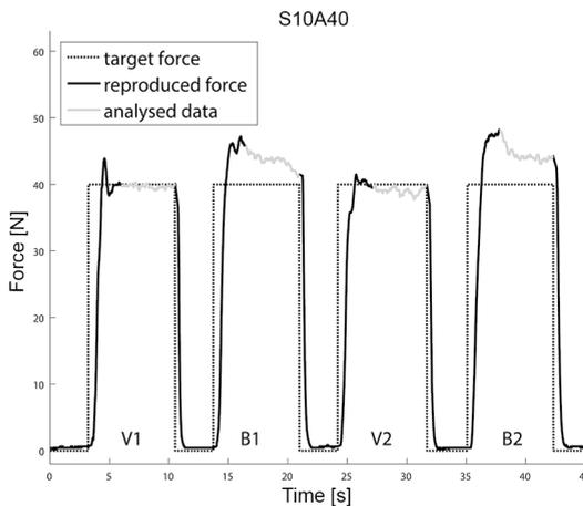
**Figure 5–3.** The raw data of the first 45 seconds of a typical trial (subject 10 – Anchor System @ 40 N) shows the target force (dotted line) of 40 N and the measured cable force (black solid line) at the back of the subject. One full trial consisted of ten visual blocks alternating with ten blind blocks (only first four blocks shown), followed by a 3 second break. The last 4 seconds of each block are used for data analysis.
