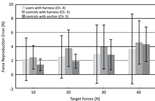
**Figure 6–2.** Force reproduction error of prosthesis users ( $n=24$ ) utilizing the traditional harness (Chapter 4), compared to that of controls ( $n=10$ ) utilizing either the harness or the anchor system (Chapter 5). The variability of the force reproduction error over the user group is larger than over the control group, which may contribute to the (statistically significant) differences *between force levels* that were present with controls, but not with users.
