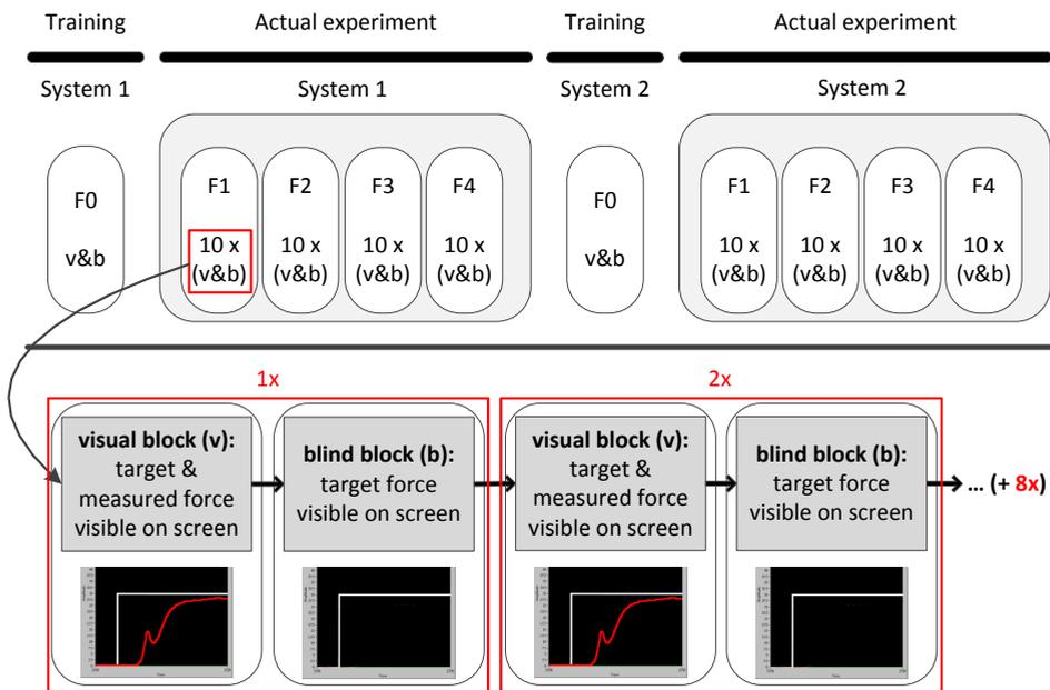
**Figure 5–2.** Flowchart illustrating the experimental procedure. Subjects performed the experiments with the two systems, Anchor System and figure-of-nine harness, with the order counterbalanced over subjects. After practicing at 15 N (F0), each system was examined at four force levels (10, 20, 30 and 40 N) during 10 visual and 10 blind blocks in alternating order. The force levels (F1 to F4) were counterbalanced over the subjects. The order of force levels differed per subject.
