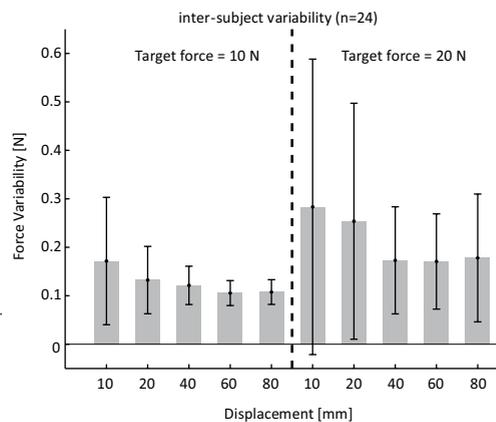
**Figure 4–10.** The force variability remains constant with increasing cable excursion for ‘cable excursion’ trials. The force variability is lower for 10 N target force than for 20 N. The bars indicate the group’s average and the whiskers the standard deviation.
