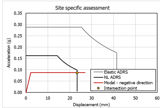
Figure 11. Site specific assessment for mode-proportional NLPO negative loading direction.
