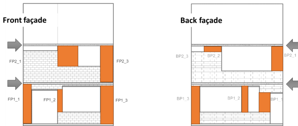
Figure 2. Piers defined on the front and back façades of Building B for positive loading.
