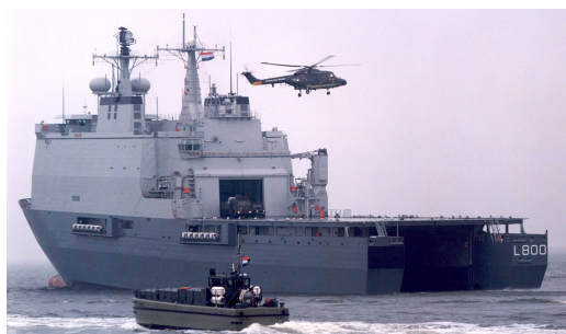
(a) LPD with helicopter deck positioned aft of the superstructure (Damen, n.d.).
