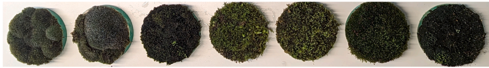
Fig. 3. Test samples (100 mm) after application of moss layer. Species from left to right: G. pulvinata (layer thickness < 10 mm), G. pulvinata (layer thickness > 15 mm), O. diaphanum , B. rutabulum , R. confertum , P. capillare , and T. muralis .
