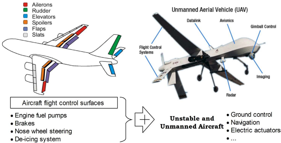
Figure 1.6: Complexity of electrical and electronic systems (E/E systems) on unstable and unmanned aircraft (adapted from [7, 20])
