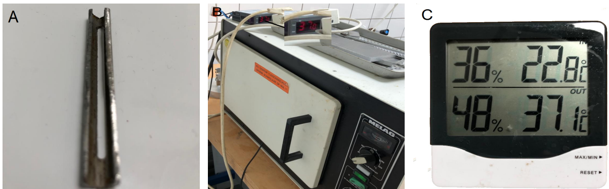
Figure 3: A) Metal mask used to placed the test soil on a constant position. B) Temperature in the oven controlled by a temperature controller (STC 1000, Ketotek, China) C) Digital thermo-hygrometer (Dostmann electronic GmbH, Duitsland)
