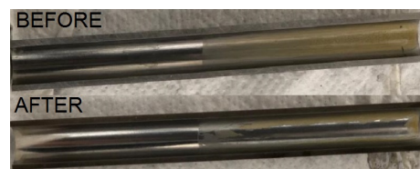
Figure 13: Before and after cleaning with a pulsating flow of 8 L/min with an amplitude of 4.5 and a frequency of 0.5 Hz
