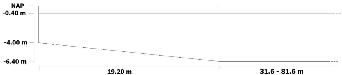
Figure 2.4 Cross section of the Amsterdam-Rijnkanaal
