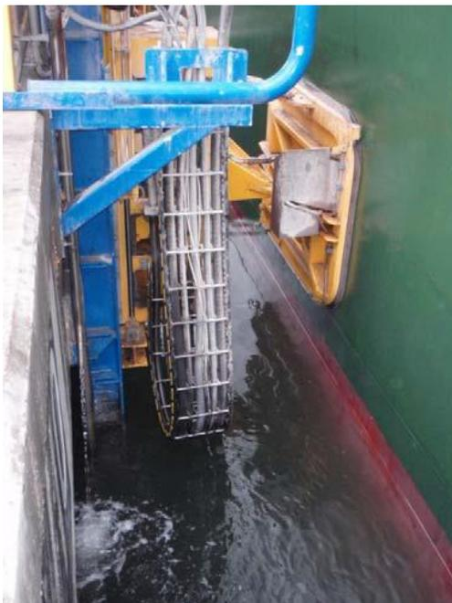
Figure 2.1 A MoorMaster™ unit connected to a ship hull
