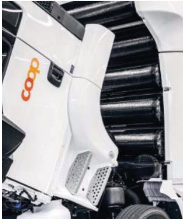
Figure 24 Positioning of the hydrogen fuel tanks in the tractor of the Coop truck behind the driver (Esoro, 2019)
