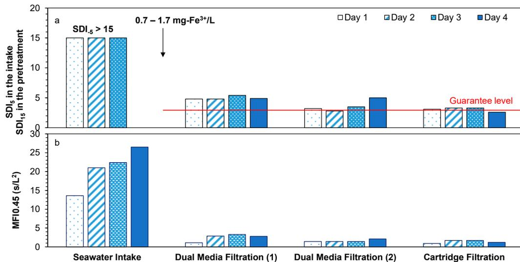
**Figure 2.** (a) Silt density index of 5 min (seawater intake) and 15 min (other samples) and (b) modified fouling index of 0.45  $\mu\text{m}$  for the SWRO pretreatment processes of the SWRO desalination plant. Chlorination was applied on day 4.
