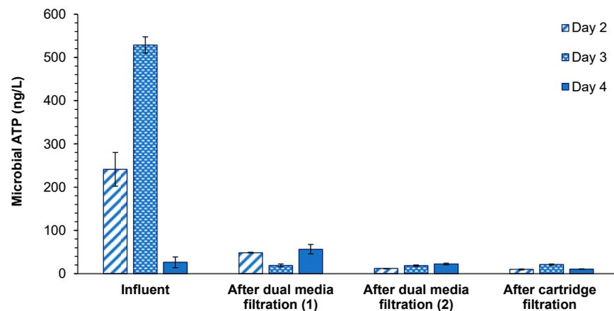
**Figure 3.** Microbial adenosine triphosphate (ATP) concentrations during the reverse osmosis pretreatment processes of the SWRO desalination plant. Chlorination was applied on day 4.
