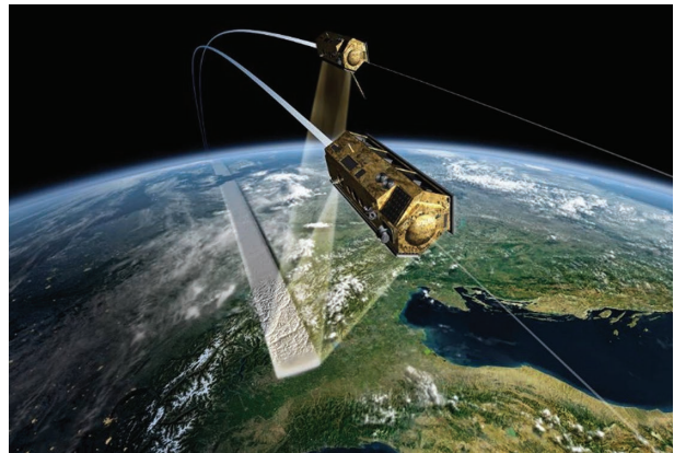
FIGURE 1. The TanDEM-X bistatic single-pass interferometric mission.
