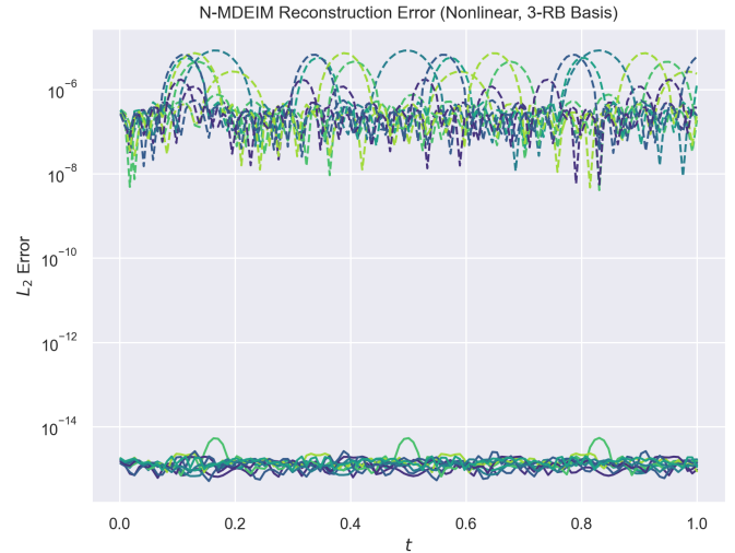
Fig. 29. Reconstruction error for the nonlinear operator evaluated with function f(x) . The basis has been obtained using the three RB solution modes ( N_{\text{full}} = 19 ). In dashed is the approximation error using a truncated basis, from which several operator modes have been removed ( N_{\text{truncated}} = 10 ). The truncated basis does not fail as drastically as the previous ones did, it simply presents a higher error, but still within an acceptable order of magnitude.
