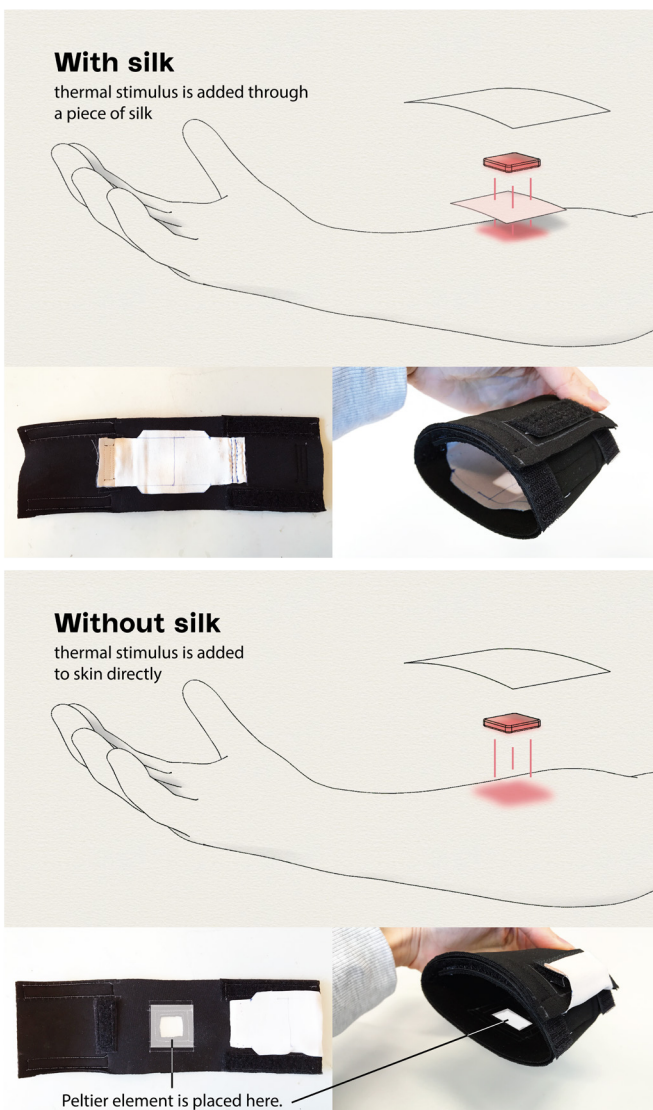
Figure 25-26. Switching between 'with silk' and 'without silk' mode by attaching the silk to the inner side or the outer side of the armband
