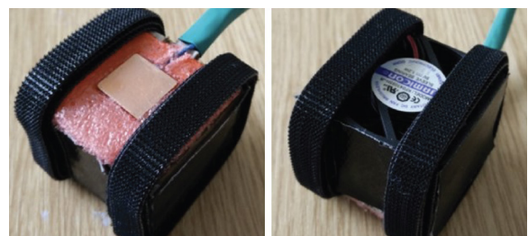
Figure 41. A fan attached to the Peltier element
