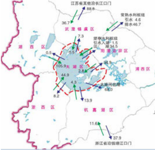
FIG. 3.21 Schematic Diagram of Water Exchange in Important Areas of Taihu Lake Basin in 2017
