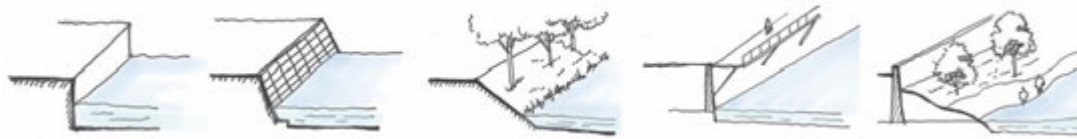
FIG. 3.164 Revetment Forms (from Left to Right): Vertical Revetment, Hard Slope Revetment, Natural Slope Revetment, Cantilever Platform Revetment, Revetment Combined with Man-Made and Nature.
