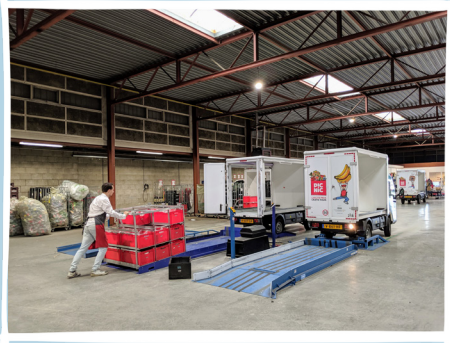
Runners placing the frame with totes in the EPV
