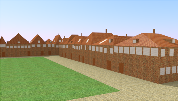
Figure 10: Example of a CityGML model generated with RANDOM3DCITY in conjunction with the existing real-world dataset of 2D footprints of buildings. This setting shows the Beestenmarkt in Delft, the Netherlands. The grammar has been adjusted to match the configuration of the buildings in that setting in order to resemble the reality as close as possible.
